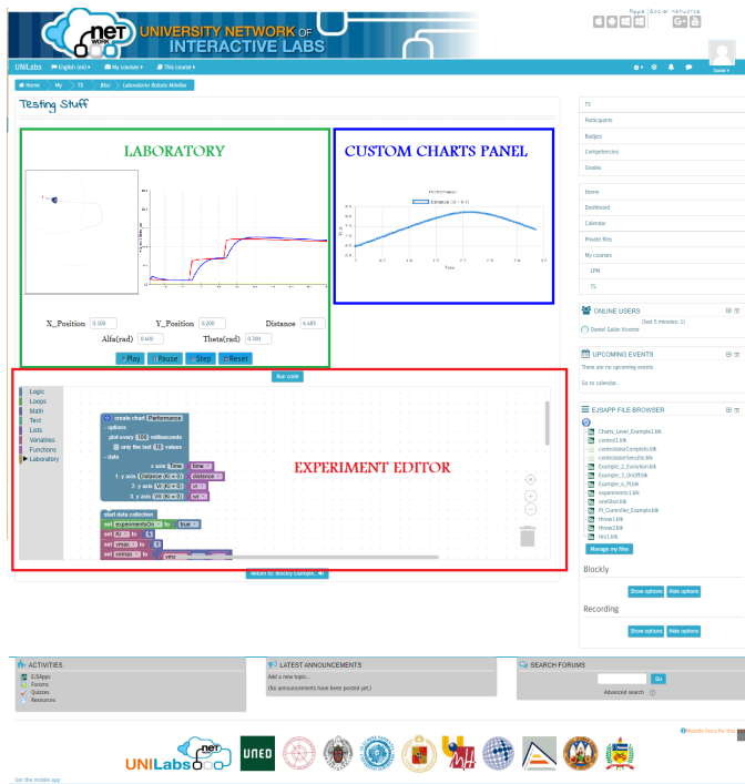
Fig. 6. Visual experimentation environment with a remote laboratory of a Furuta Pendulum to perform Control experiments
