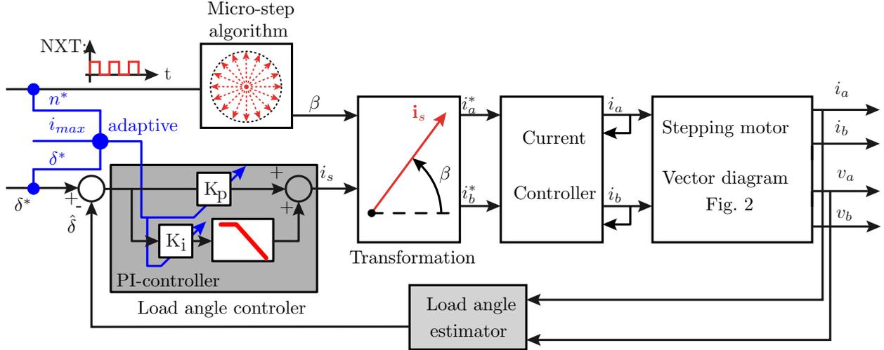
Fig. 3. Typical stepper motor drive principle where current vector  $\mathbf{i}_s$  position  $\beta$  is determined by step command NXT pulses sent by the user extended with adaptive PI load angle controller
