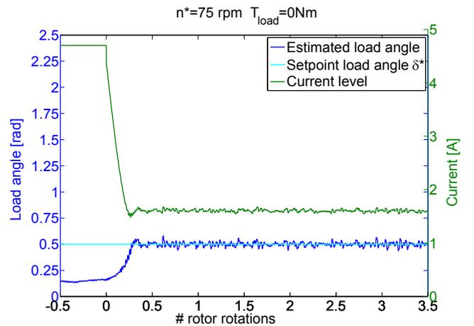
Fig. 6. Controlled current reduction and load angle optimisation at low speed and unloaded
