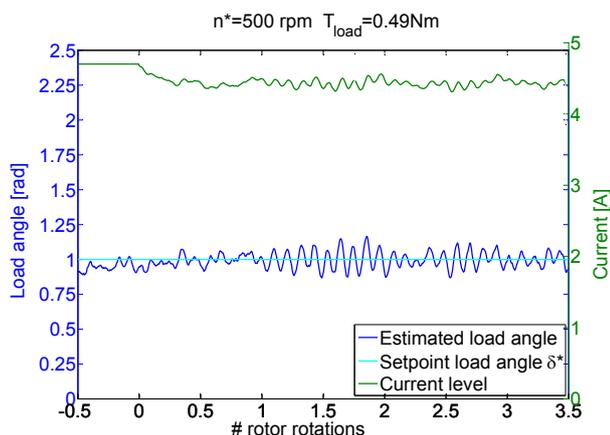
Fig. 8. Controlled current reduction and load angle optimisation at high speed and fully loaded motor
