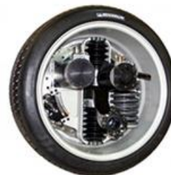
Fig. 1. Active wheel from Michelin.
