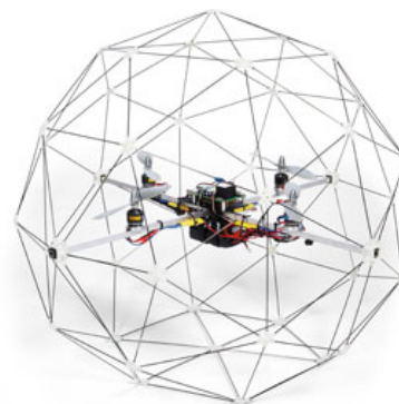
Fig. 1. The Quanser Qball-X4 quadrotor UAV
