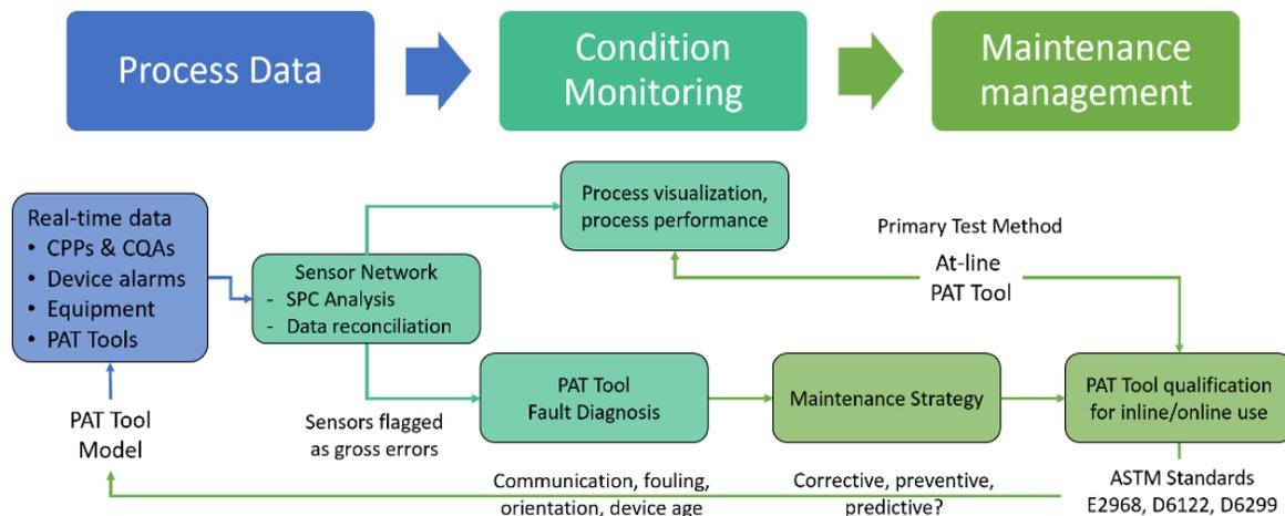
Figure 2: Integrated maintenance management for instrumentation systems in continuous pharmaceutical mfg.
