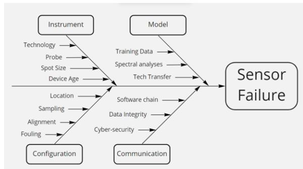
Figure 1: Potential failure sources of process analyzers
