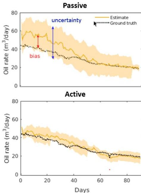
Figure 2. Production surveillance result of one of the eight wells using the two sensing approaches. The estimated rates using the passive sensing approach exhibit higher bias and uncertainty (with respect to the ground truth) compared to the active sensing approach. In addition, active sensing required 25 fewer well tests than its counterpart.
