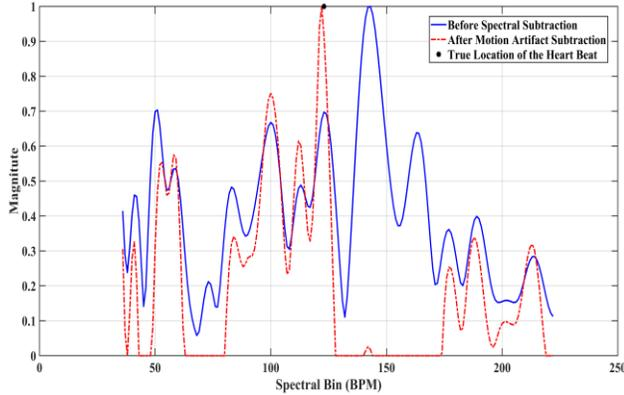
Figure 1. Spectrogram of the original PPG signal (solid line), spectrogram of the processed signal (dashed-dotted line), and location of the true heartbeat frequency (bullet marker).
