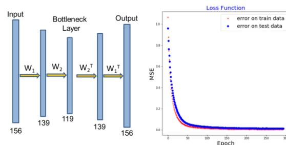
Figure 1. Optimized DAE Architecture and Model Training Process
