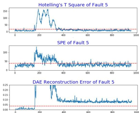
Figure 3. Process Monitoring with Hotelling's  $T^2$ , SPE and DAE in case of Fault 5
