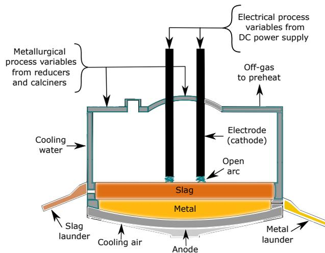
Figure 1: Direct current electric arc furnace
