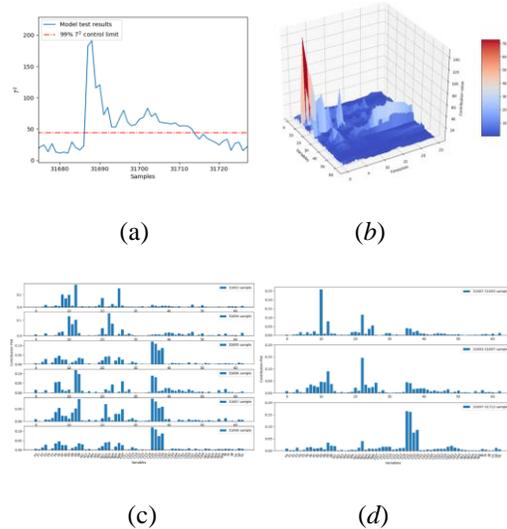
Figure 3. Fault diagnosis based on accumulated Hotelling Statistic
