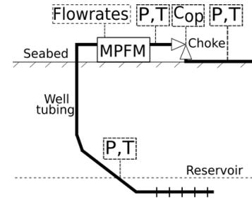
Figure 1 – Schematic representation of a well with available measurements.
