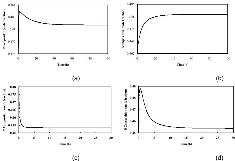
Figure 3. The open-loop responses of the RDC-TBER. (a) C composition for CSI, (b) D composition for CSI, (c) C composition for CSII(CSIII), (d) D composition
