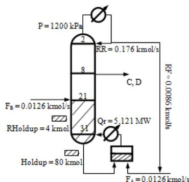
Figure 2. Process synthesis and design of RDC-TBER
