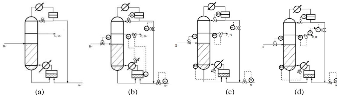
Figure 1. RDC-TBER and its control system designs: (a) RDC-TBER, (b) CSI, (c) CSII, (d) CSIII
