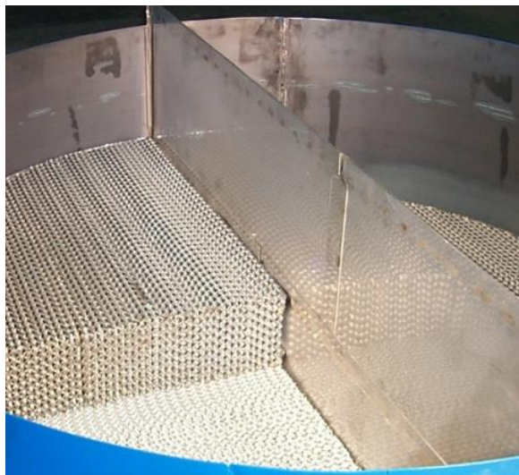
Fig. 3 Loose dividing wall column for a revamp project of a conventional column to a dividing wall column.
