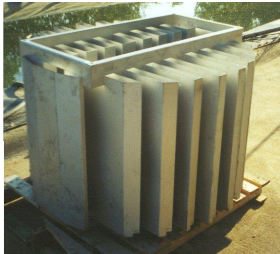
Figure 5. FRI VKG Trough Type Liquid Distributor
