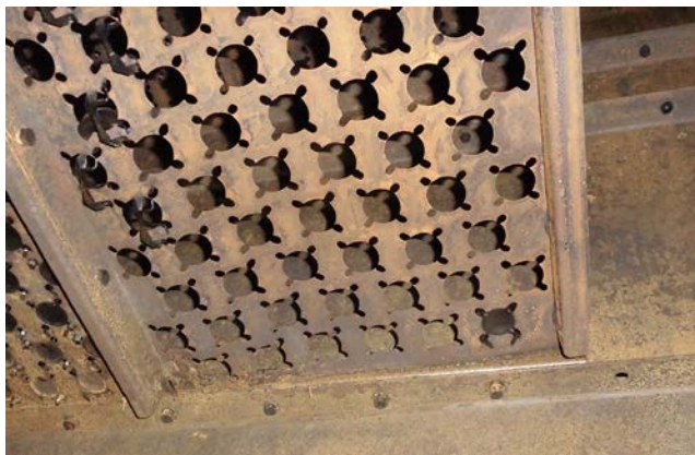
Fig. 5a: Panel with lost caged valves
