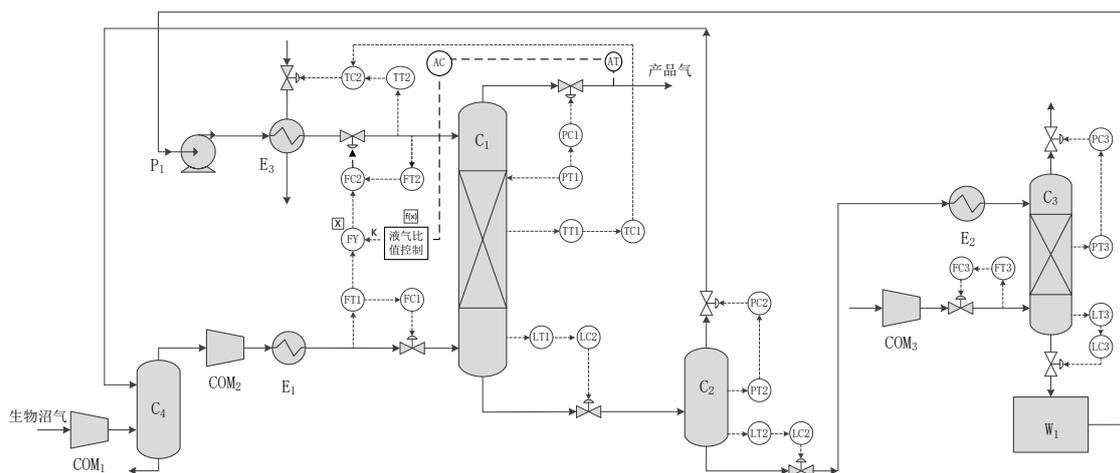
Fig. 3 Flow sheet of dynamic simulation of supervisory control scheme
