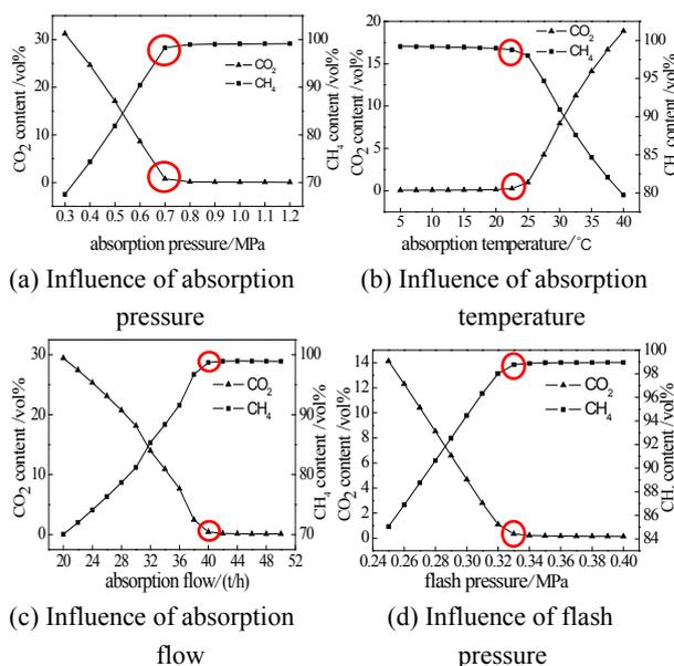
**Fig.2 Influence of different operation parameters on purification effect**
