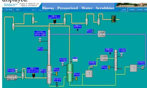
Fig.9 Process monitoring system on WINCC
