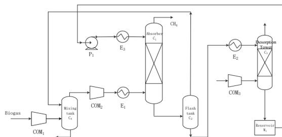
Fig.1 Flow sheet of pressurized water scrubbing
