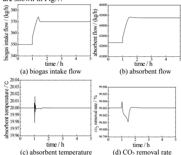
Fig.7 Dynamic response curve after lifting system load
