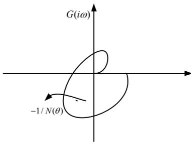
Fig. 4. The oscillation criterion on the Nyquist diagram.
