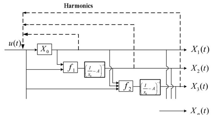
Fig. 5. Block diagram for the numerical computation of functional expansions.
