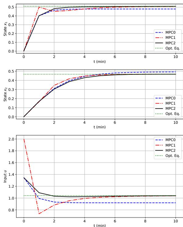
Fig. 1. Comparative closed-loop results using the three controllers: states (top and middle) and input (bottom).
