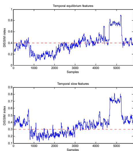
Fig. 5. Online CPM for one fault case (data set 1.1) based on two types of temporal features
