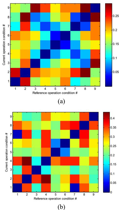
Fig. 2. DISSIM index between any two operation conditions for (a) temporal equilibrium features and (b) temporal slow features.
