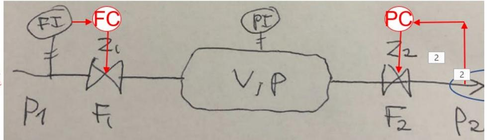
Comment: One may think that it does not work since  $p$  is left uncontrolled, which may lead to blow-up of the pipeline. However, the fact that  $p$  is uncontrolled does not by itself mean that we have a problem. In most cases, pressures are left uncontrolled as we rely on self-regulation, for example, valve 2 may be kept fully open to minimize pressure drop. Thus, the problem is not that  $p$  is left uncontrolled, but rather that  $p_2$  is controlled.
