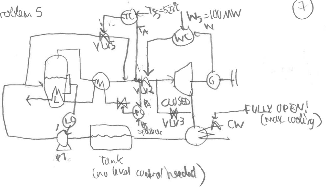
(a)  $MV = \begin{bmatrix} VLV1 \\ VLV2 \\ VLV3 \\ VLV4 \\ VLV5 \\ P1 \end{bmatrix} = \begin{bmatrix} \text{Hot gas feed} \\ \text{Steam valve} \\ \text{Bypass steam} \\ \text{CW} \\ \text{Bypass water} \\ \text{Pump} \end{bmatrix}$
