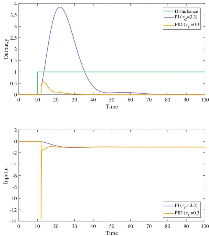
Figure 7: Output response to a step disturbance of magnitude 1 for PI (purple) and PID (orange)
