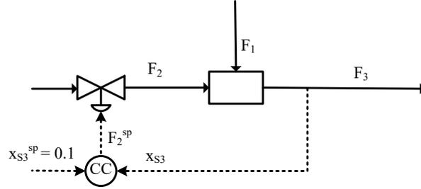
Figure 8: Control structure for the nominal point
