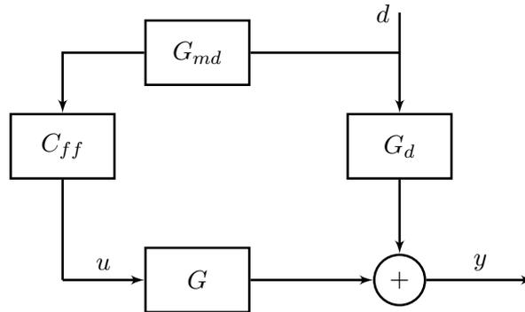
Figure 1: Block diagram for feedforward control
