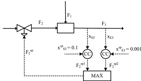
Figure 9: Control structure that handles both the nominal and the extreme cases
