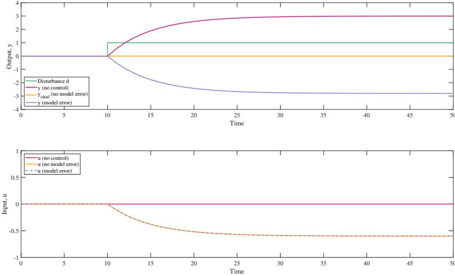
Figure 2: Comparison of step response for open loop, feedforward with no model error and feedforward with model error.
