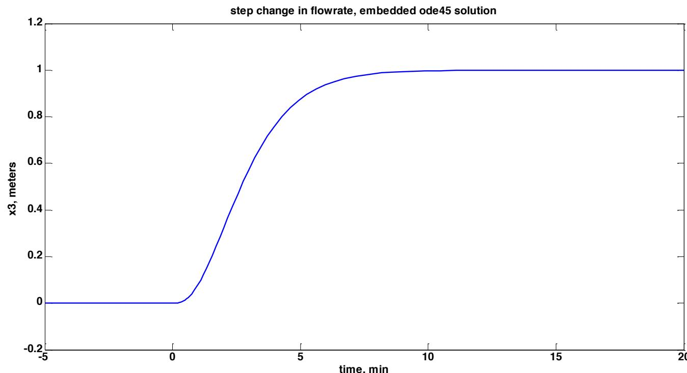
4. Write a script file (m-file) with a for-loop with ode45 used to integrate the function file from time = -5 minutes to time = 20 minutes, *with a sample time of 0.5 minutes*. Again, allow the input to change from 0 to 1 at t = 0 minutes, and compare your results with problems 2 and 3.
