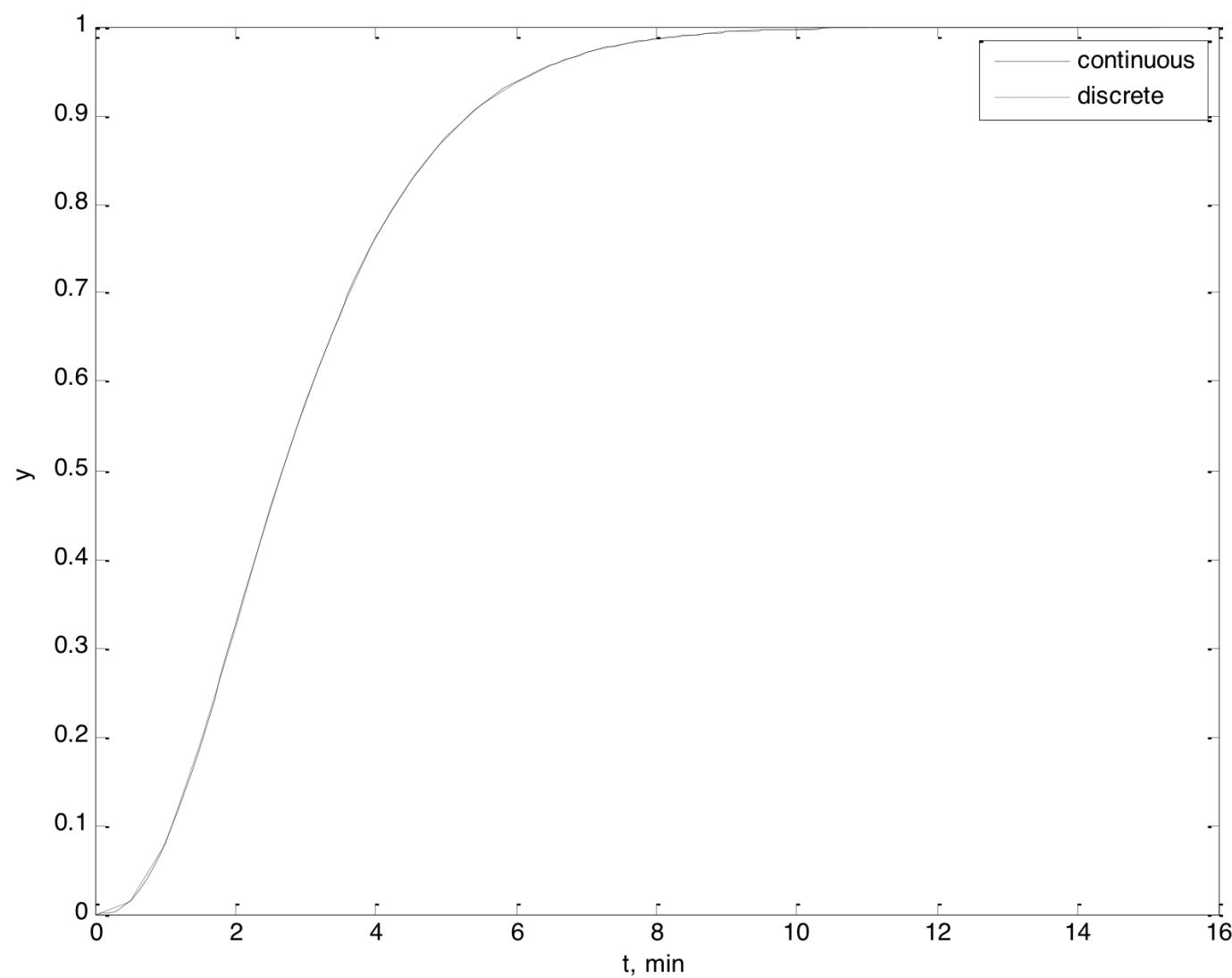
2. Design a digital *PID controller* with a sample time of 0.5 minutes. Use a continuous representation of the *plant* for simulations (using `ode45`), but implement a discrete controller on the simulated plant that you developed in Homework 1. The initial conditions for the input and output (and all states) are 0. Make a setpoint change to a value of  $r = 1$  at  $t = 1$  minute.
