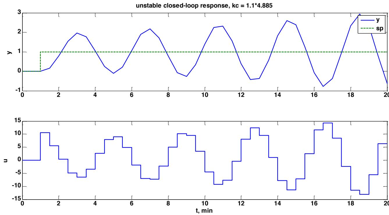
Notice that the output plots are somewhat “jagged.” In the m-file I show how to plot additional time points between the sample time to make the output curves look smoother, as shown in the plot below.
