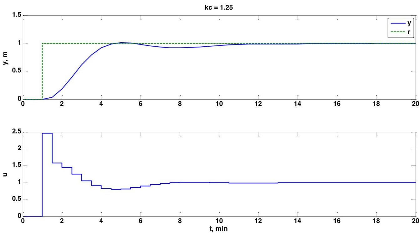
3. Now, adjust  $k_c$  until the closed-loop system enters a continuous oscillation, on the verge of instability (constant amplitude output and manipulated input). Calculate the discrete closed-loop poles for this value of  $k_c$ . Is this result consistent with your simulation results?
