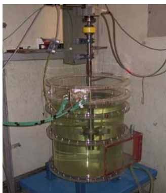
A stirred tank used for studies of heat transpt and flow phenomena.
