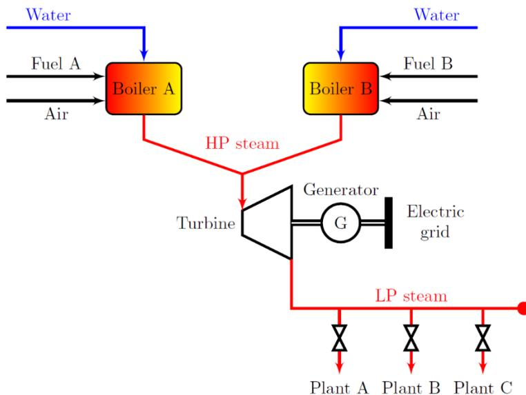
Figure 1 shows a simplified flowsheet of the system. Here, two boilers generate high pressure steam by burning different fuels, Fuel A and Fuel B respectively. The high pressure (HP) steam is expanded to low pressure (LP) in a turbine which drives a generator to produce electric power to the grid. The low pressure steam is distributed through a steam network to each consumer (Plant A, B,C).
