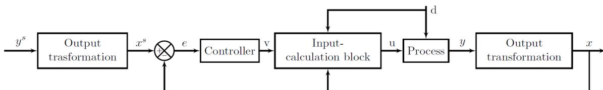
*Figure 1 Block diagram of a control structure with embedded process knowledge through input and output transformation.*
