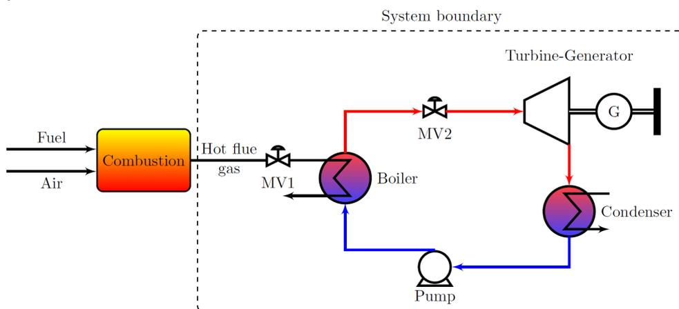
*Figure 1 Simplified heat-to-power cycle flowsheet. The dotted line shows the boundary of the system (steam side).*
