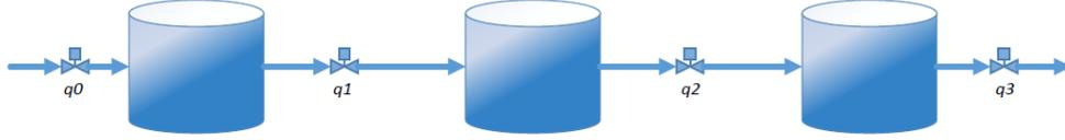
Figure 6: The process which is modeled in this project. The levels + TPM are the CVs while the four flows are the MVs.
