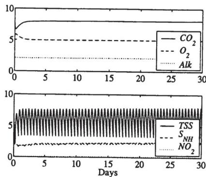
Fig. 4. Simulated concentrations in the fish tanks (oscillations caused by twice daily feeding).
