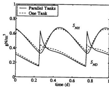
Fig. 3. Ammonium and soluble organic nitrogen in the fish tank effluent.
