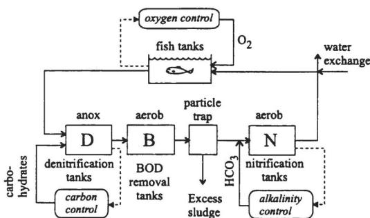
Fig. 1. A schematic picture of a RAS with control.
