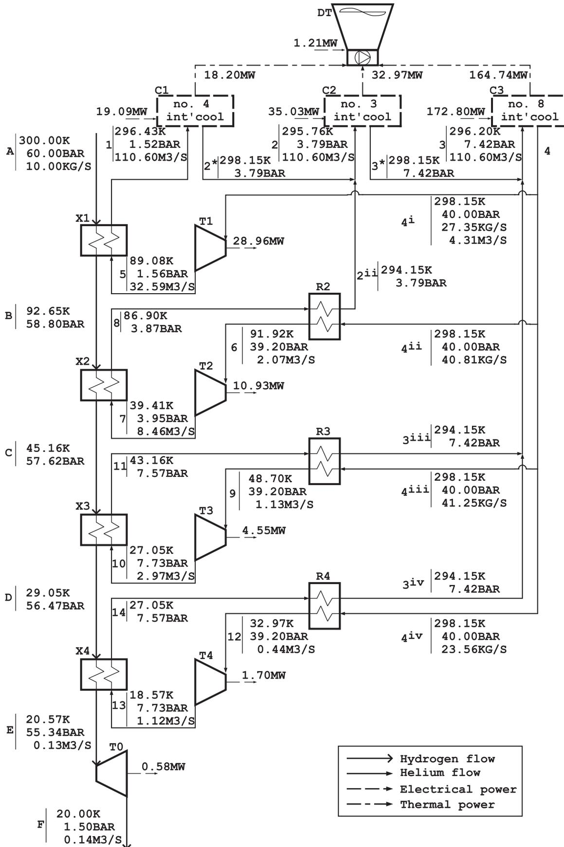
Fig. 1 – Layout of the plant detailed with results of temperature, pressure and mass flow rate for hydrogen and helium flows; volumetric flow rate and electric power for compressors, expanders and dry cooling towers.
