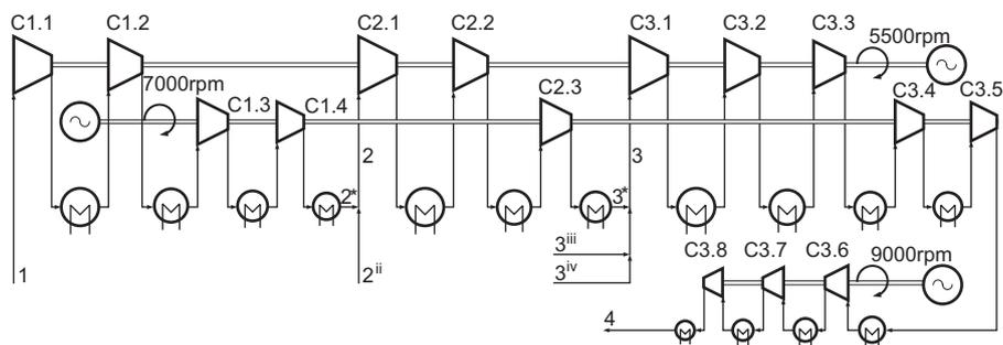
Fig. 2 – Layout of the 15 intercooled compressors showing the adopted three-shaft arrangement and the chosen rotation speeds.
