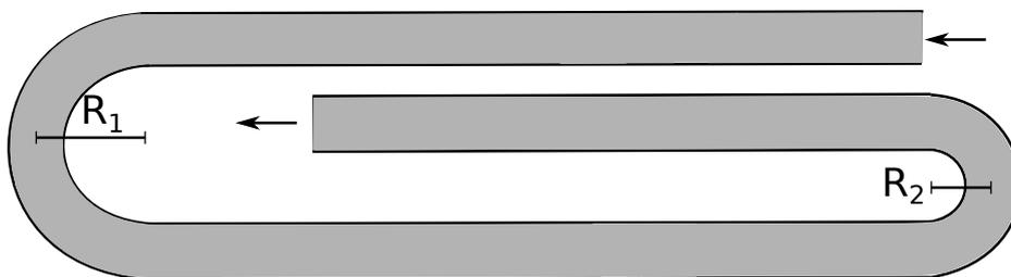
**Figure 3:** Pipe separator with two turns with radius  $R_1$  and  $R_2$  resulting in centrifugal forces being introduced.
