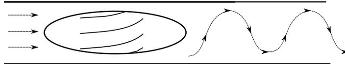
**Figure 4:** Swirl element. The flow enters the separator and a static swirl element introduces an angular velocity causing the fluid to have a swirling flow through the separator.
