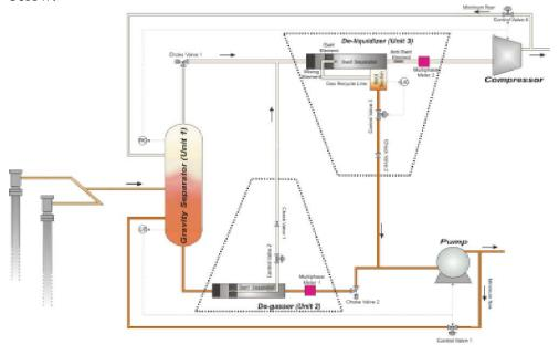
In this process liquid and gas coming from a well are to be separated, and the separation is done in two stages, where first the bulk separation is done in the Gravity separator, and then the gas-rich phase is sent to the deliquifier, and the liquid-rich phase is sent to the degasser.
