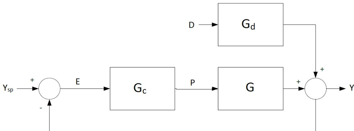
Figure 1: Block diagram of a control system with a PI controller [6].
