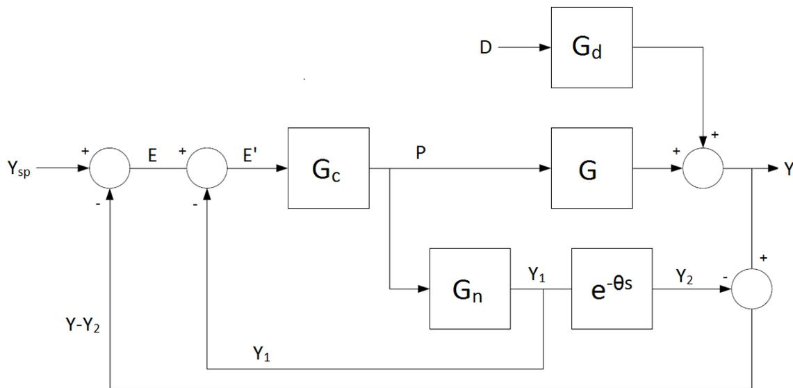
Figure 2: Block diagram for a process with the Smith predictor controller [6].
