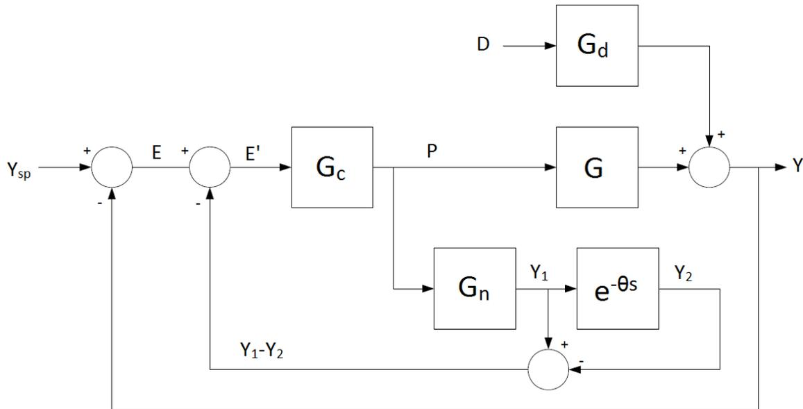
Figure 3: The Smith Predictor block diagram re-drawn as two nested feedback loops [6].
