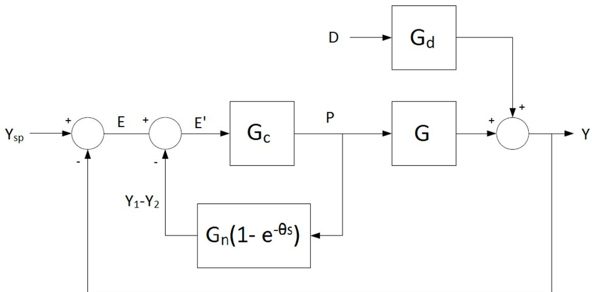
Figure 4: The Smith Predictor block diagram drawn in reduced form [6].
