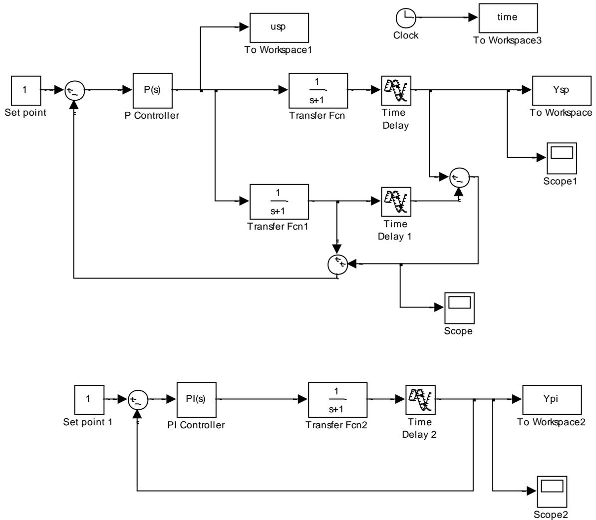
Figure 5: Block diagram of the Smith predictor and PI controller created in Simulink. The top block diagram is the Smith predictor structure and the bottom one is for a process with PI control.
