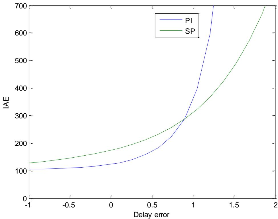
**Figure 20: IAE plotted against the delay error for case 2 with the process  $g=\exp(-s)/(8s+1)$  when the optimal tuning is applied in both controllers.**
