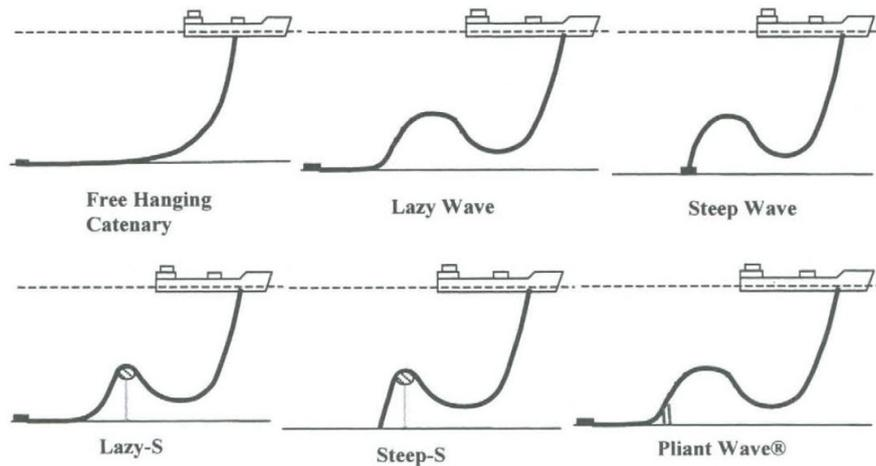
Figure 1.4: An overview of different riser configurations
