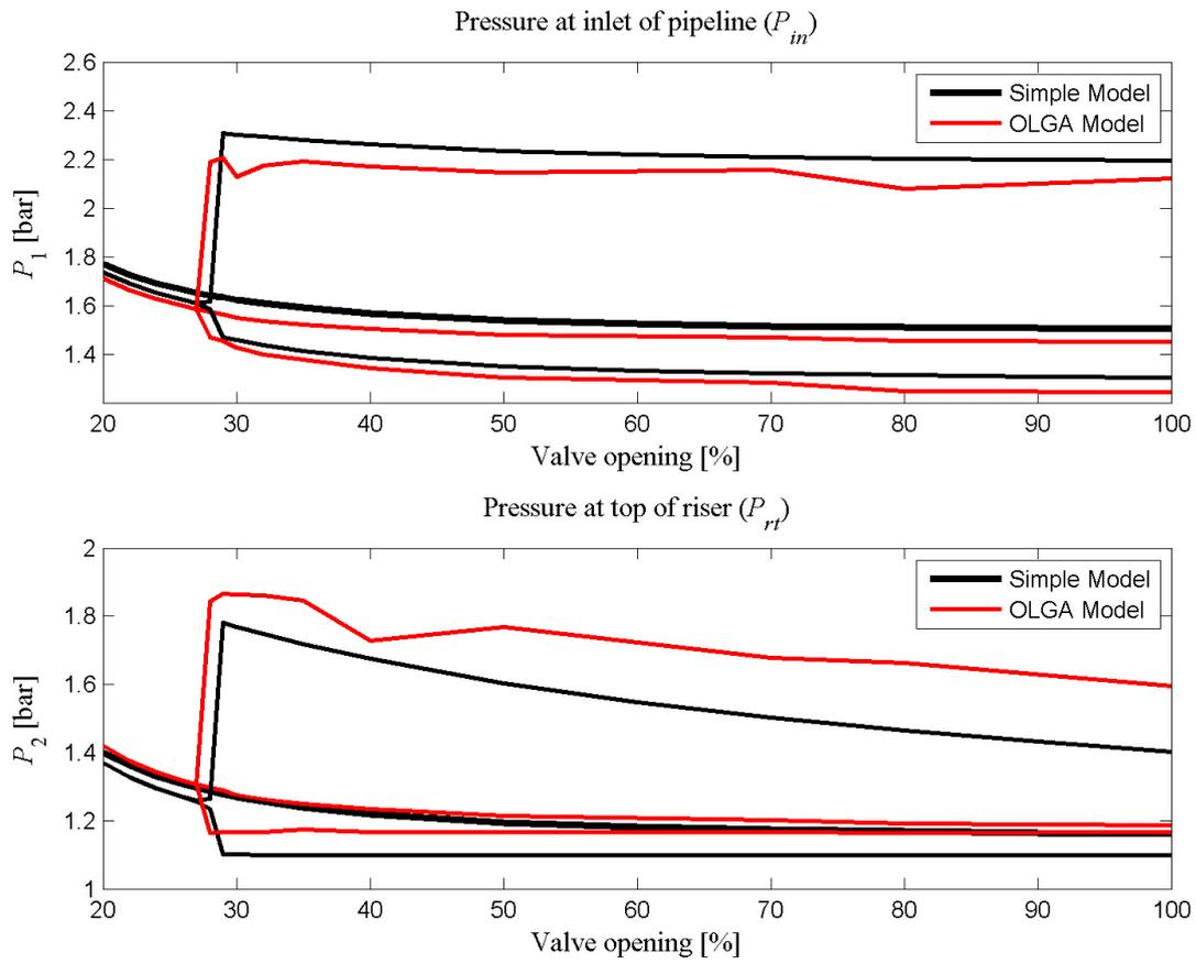
**Figure 5.10:** Simulation data from S-shaped riser case in OLGA compared to the simple model for a L-riser
