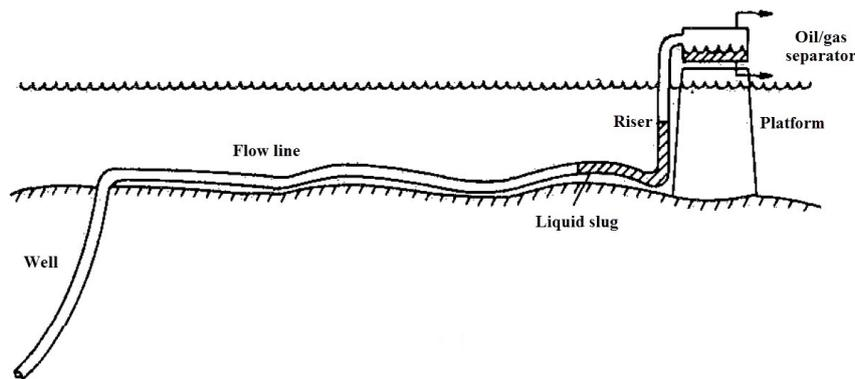
Figure 1.1: A common riser configuration
