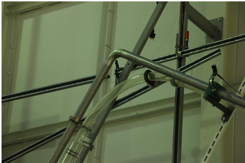
**Figure 3.5:** The bend in the steel pipe compared with the bend in the acrylic pipeline
