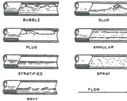
Figure 1.2: Flow patterns occurring in a horizontal pipeline
