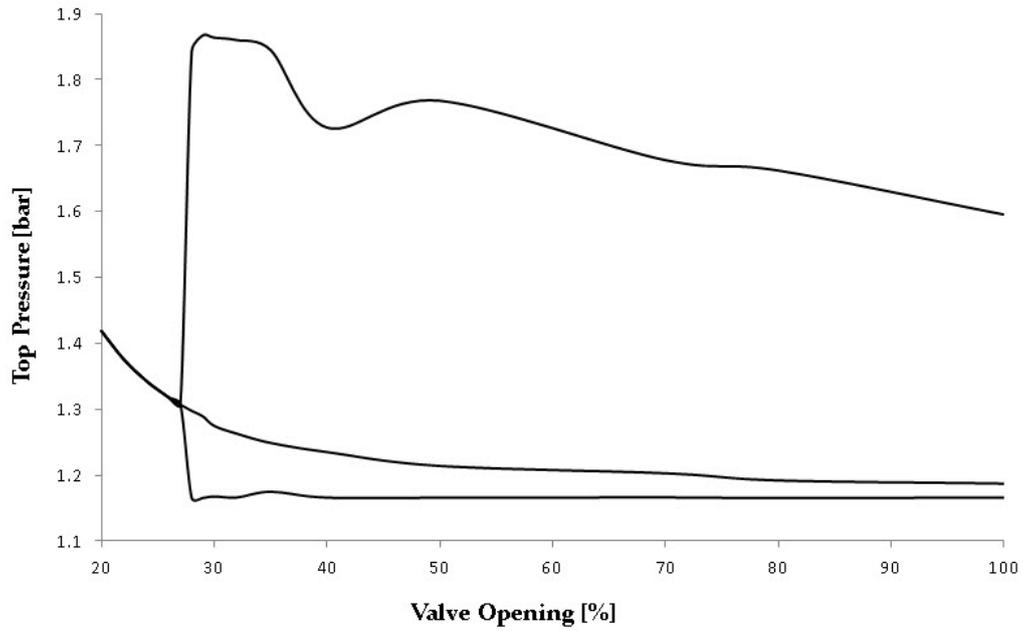
Figure 5.4: Bifurcation diagram made with simulation data from OLGA showing the variations in top pressure over a range of choke valve openings
