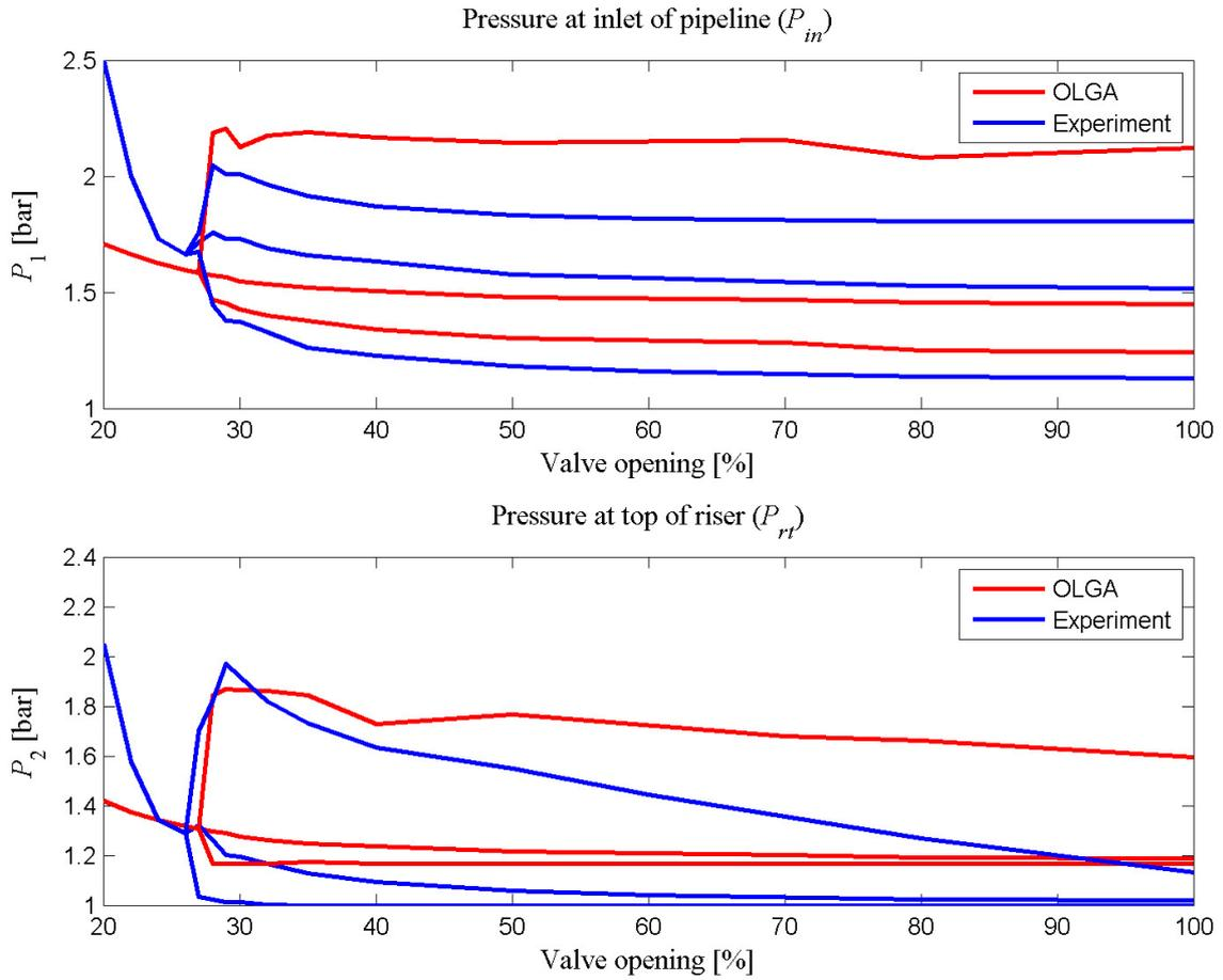
**Figure 5.11:** Simulation data from S-shaped riser case in OLGA compared with experimental results from a S-shaped riser
