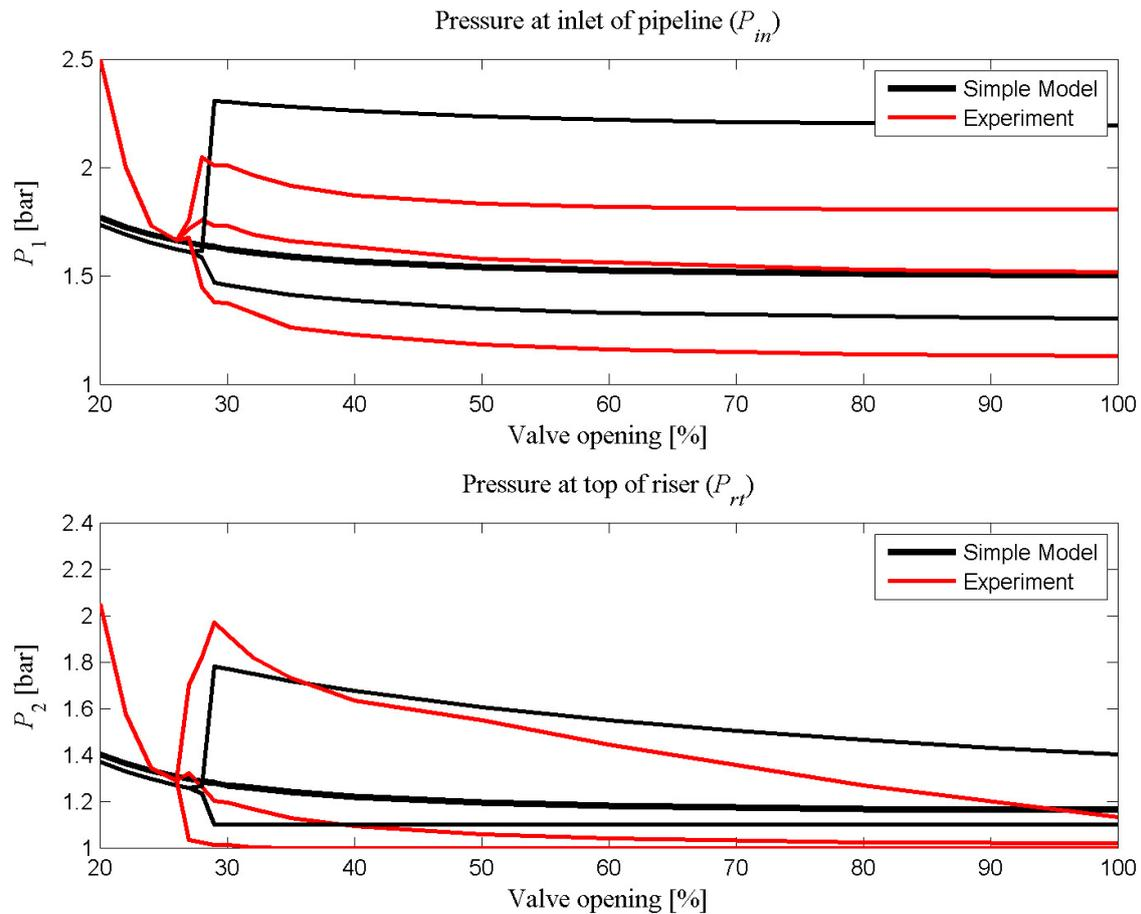
**Figure 5.12:** Simulation data from the simple L-shaped riser model compared with experimental results from a S-shaped riser
