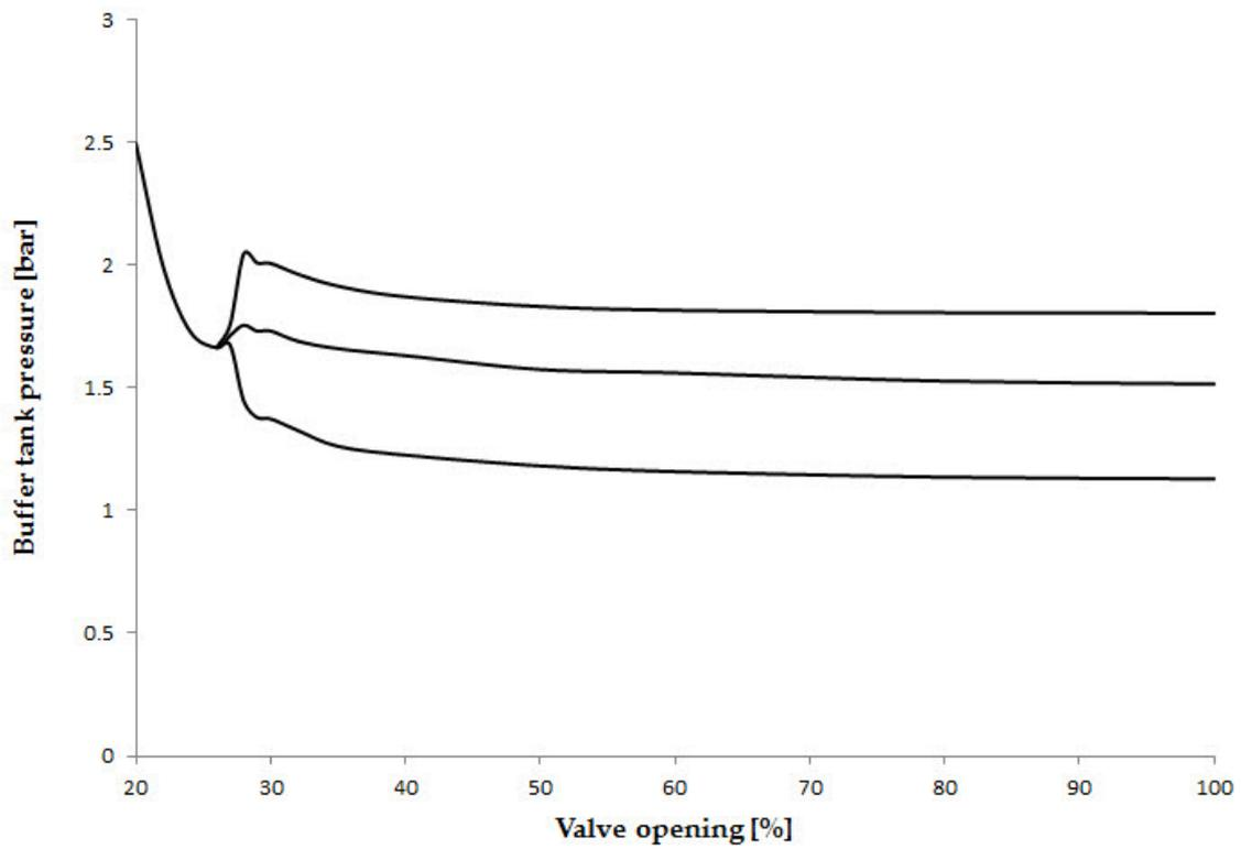
Figure 5.7: Bifurcation diagram showing how the buffer tank pressure changes with valve opening
