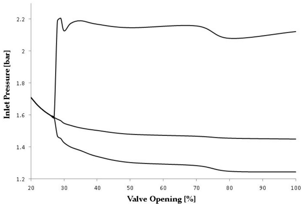
Figure 5.3: Bifurcation diagram made with simulation data from OLGA showing the variations in inlet pressure over a range of choke valve openings
