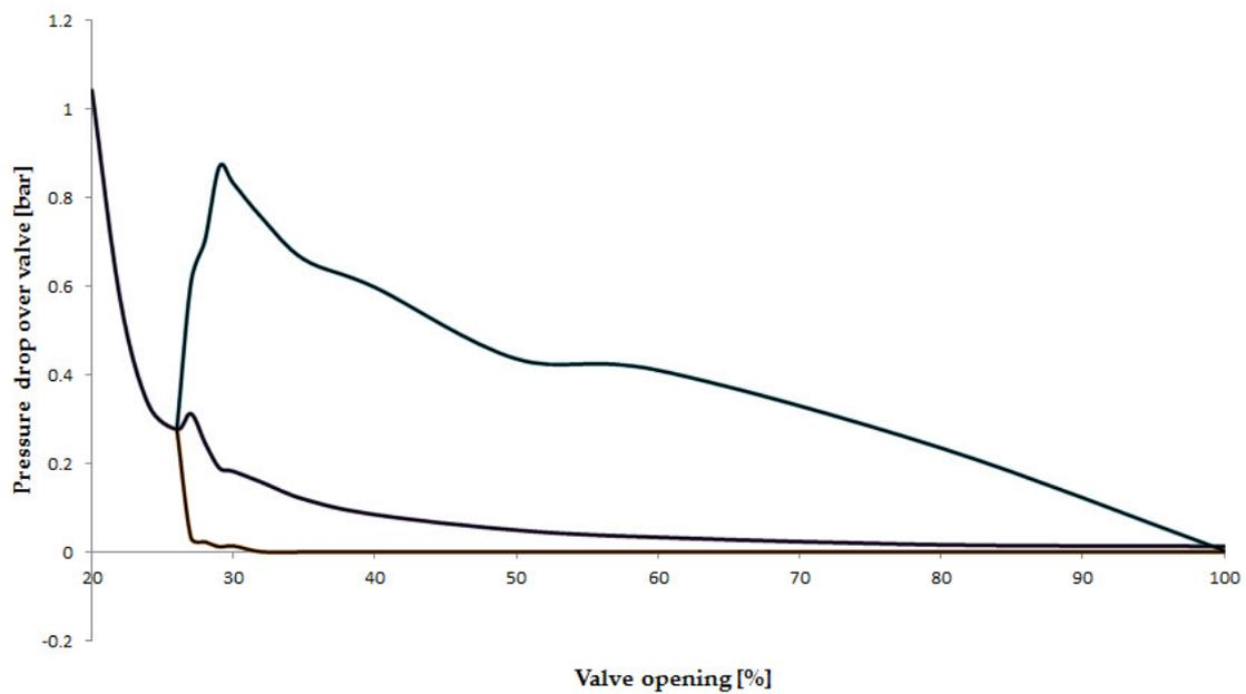
Figure 5.8: Bifurcation diagram showing how the pressure drop over valve changes with valve opening
