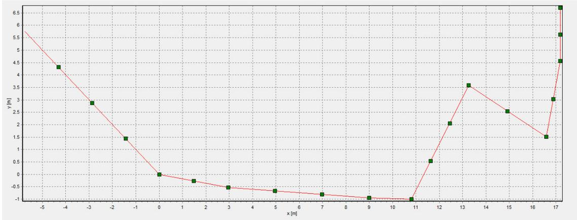
**Figure 2.1:** The geometry of the s-riser in Olga
