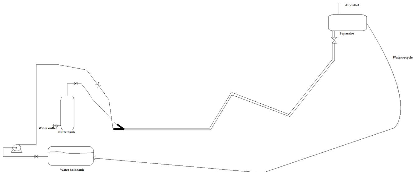
**Figure 3.1:** A simplified flow diagram of the experimental set up
