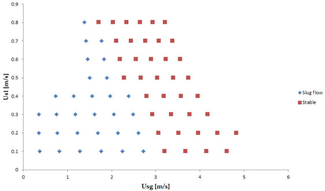
Figure 5.2: Stability map achieved using the simplified simulation case in OLGA
