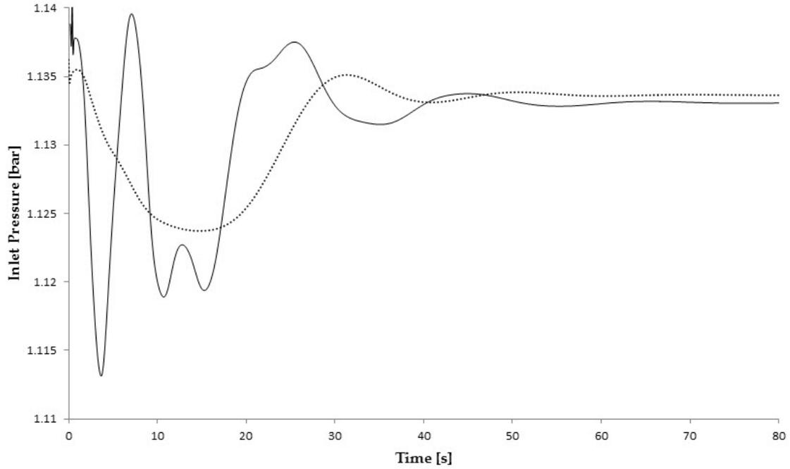
**Figure 2.3:** The Differences between isothermal simulation (solid line) and non-isothermal simulation (dotted line)
