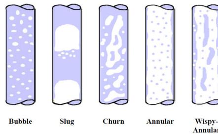
Figure 1.3: Flow patterns occurring in a vertical pipeline
