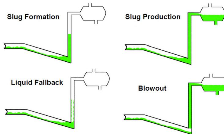
Figure 1.5: The mechanism of slug formation
