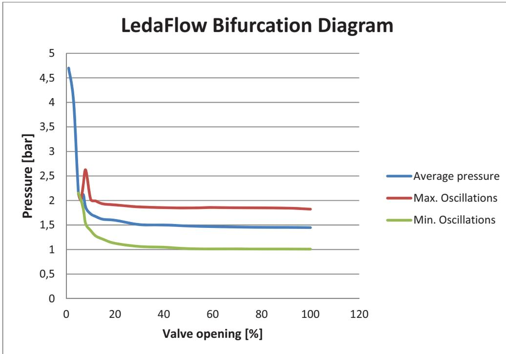
Figure 39: Bifurcation diagram of Buffer pressure- based on LedaFlow Simulations
