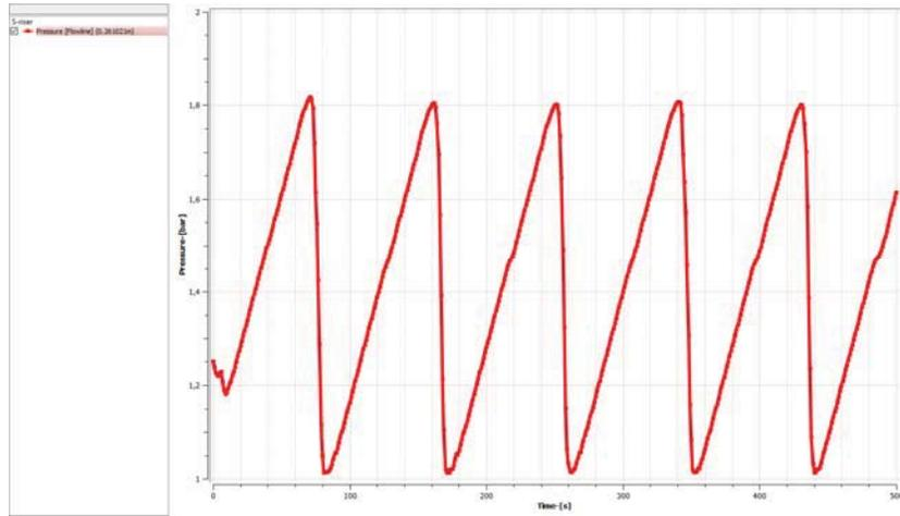
Figure 32: Pressure Oscillations in Severe Slugging I (SSI) region
