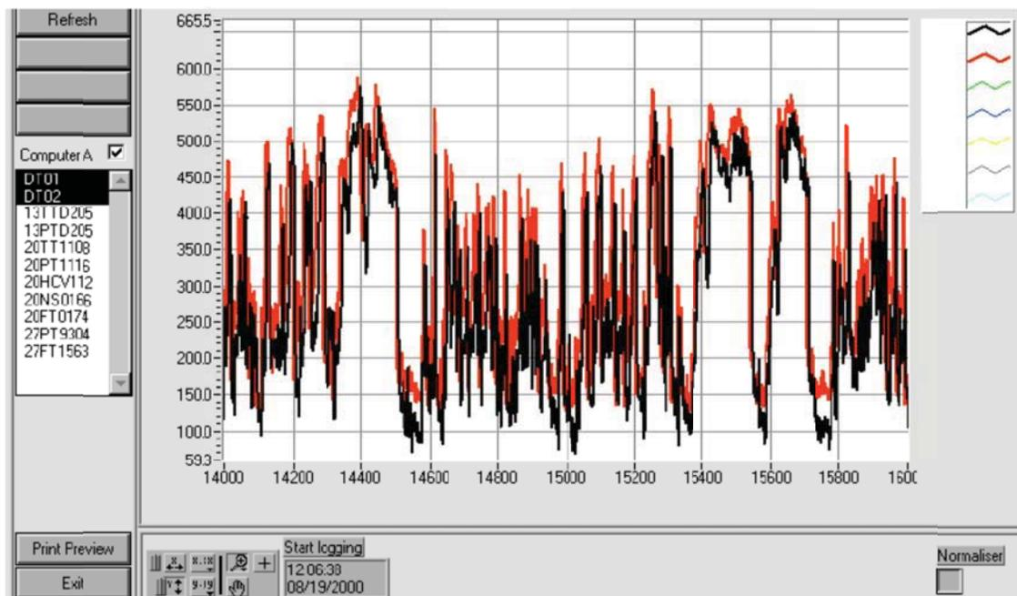
Figure 5: Recording of Severe-slugging in North Sea
