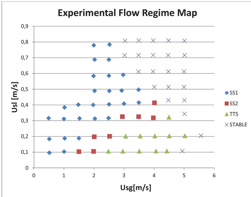
Figure 36: Obtained Flow regime map for Steel S-riser based on Experiments
