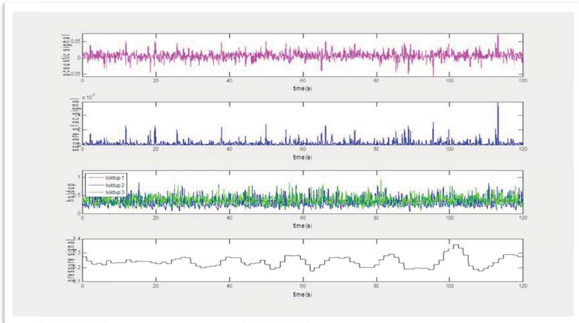
Figure14: Acoustic, Holdup and Pressure Signals for Stable Flow. (Source: [6])
