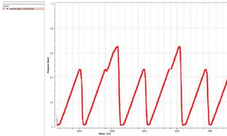
Figure 33: Pressure Oscillations in Severe Slugging II (SSII) region
