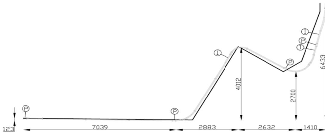
Figure 16: S-riser geometry (lengths are in millimeters). (Source: [10])
