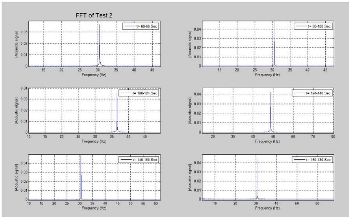
Figure 31: Fast Fourier Transform of acoustic signal with a change in valve opening percent from 25 to 20
