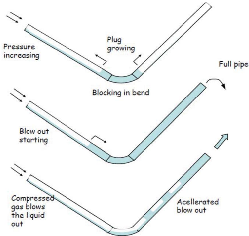
Figure 4: Severe slugging principle (Source: [4])
