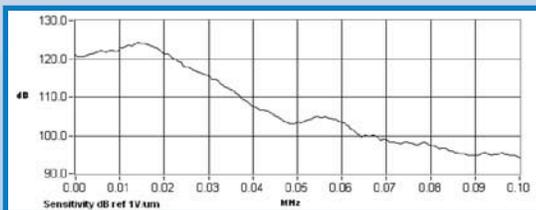
Frequency response of R1.5I. Calibration based on ASTM E 1106.
