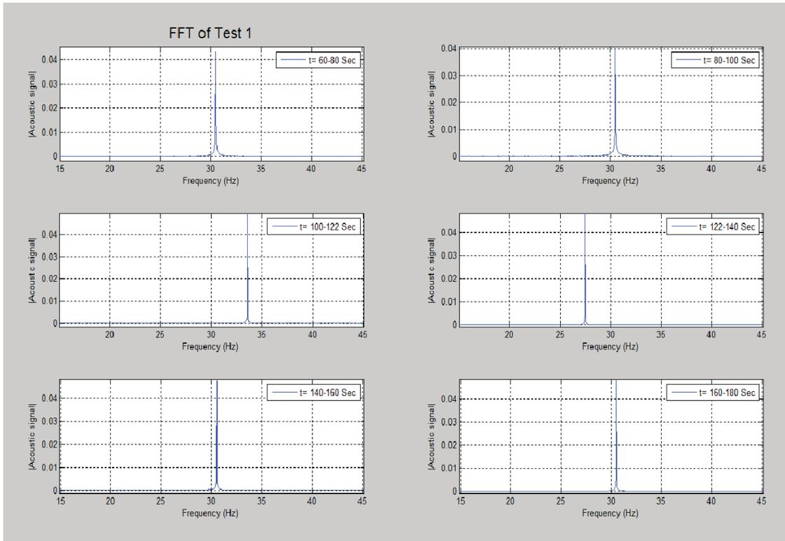
Figure 30: Fast Fourier Transform of acoustic signal with a change in valve opening percent from 20 to 25
