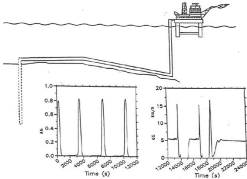
Figure 6: Steady flow after severe slugging, (Source: [3])
