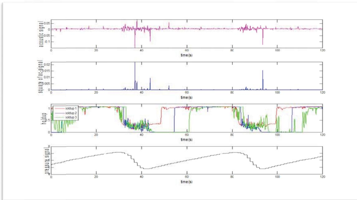
Figure 13: Acoustic, Holdup, and Pressure Signals for SS1. (Source: [6])
