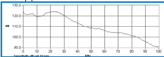
Frequency response of R.451. Calibration based on ASTM E 1106
