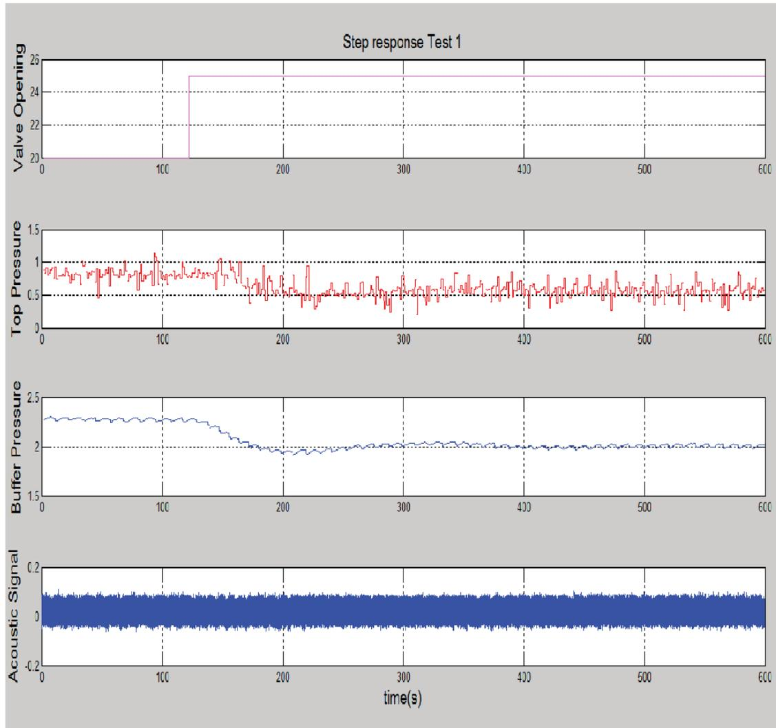
Figure 28: Step response of pressure and acoustic sensors with a step change in valve opening from 20 to 25 percent
