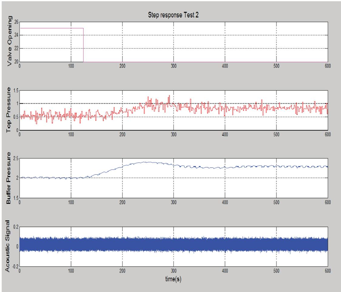
Figure 29: Step response of pressure and acoustic sensors with a step change in valve opening from 25 to 20 percent
