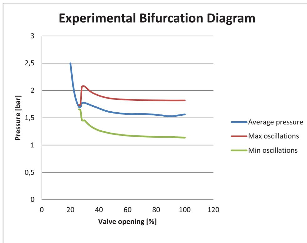
Figure 38: Bifurcation diagram of Buffer pressure- based on Experiments
