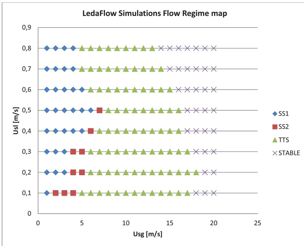
Figure 37: Obtained Flow regime map for Steel S-riser based on LedaFlow Simulations
