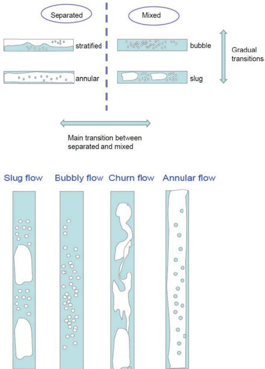
Figure 2: different flow regimes in horizontal and vertical pipelines
