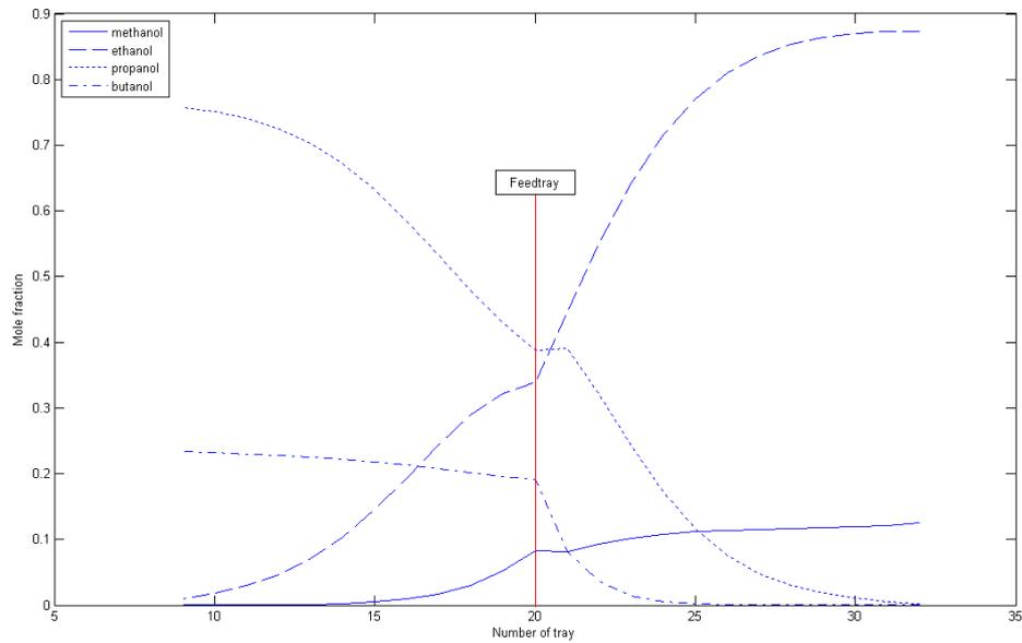
Figure 13: Optimal separation in the prefractionator
