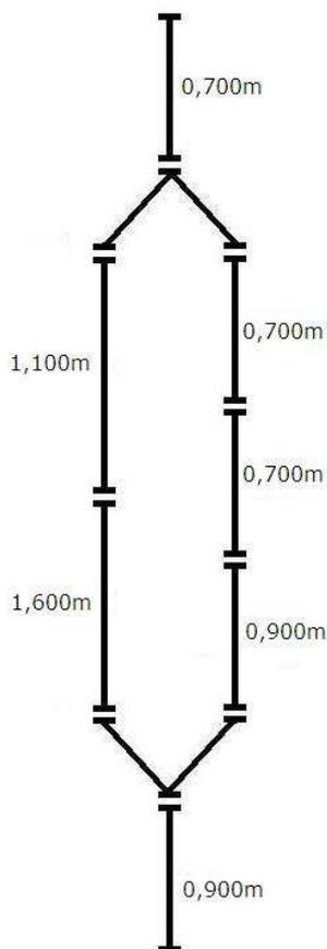
The height of the section between  $S_1$  and  $S_2$  is 0,7 metres. The H.E.T.P. of this section is thus:
