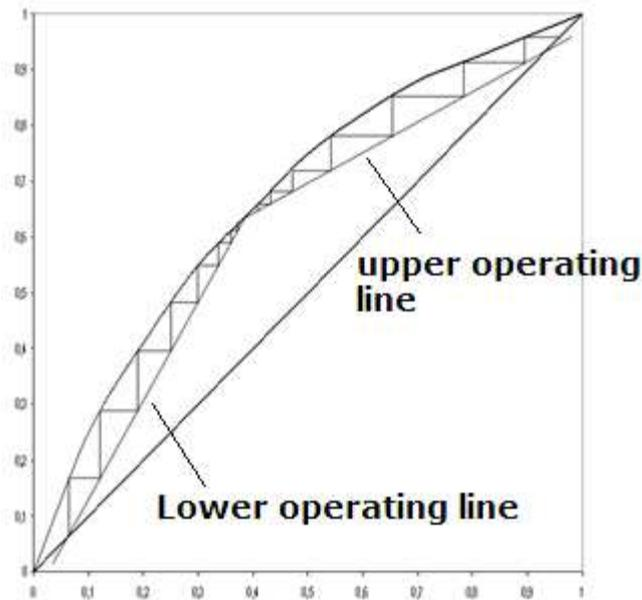
Figure 2: VLE with operating lines
