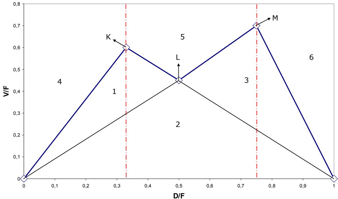
Figure 4: Minimum energy diagram for a 3-component mixture
