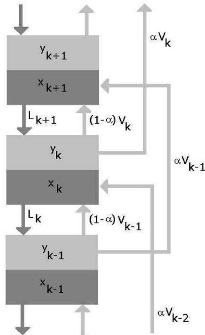
Figure 3: Vapour bypass
