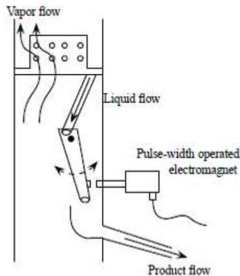
Figure 17: Electromagnetic funnel
