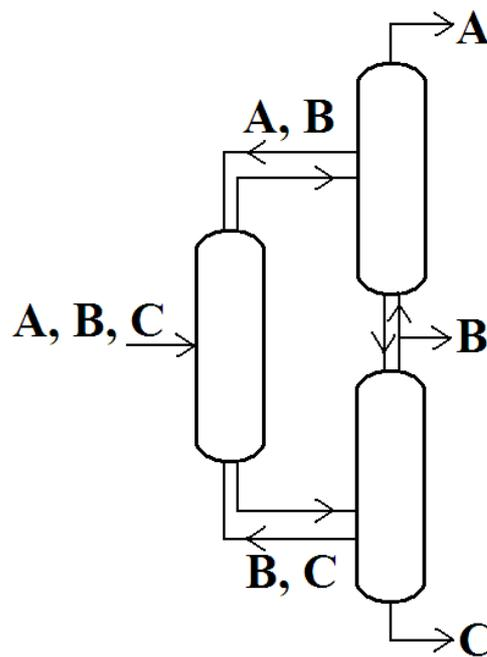
Figure 10: Petlyuk arrangement
