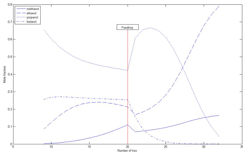
Figure 14: Non optimal separation in the prefractionator
