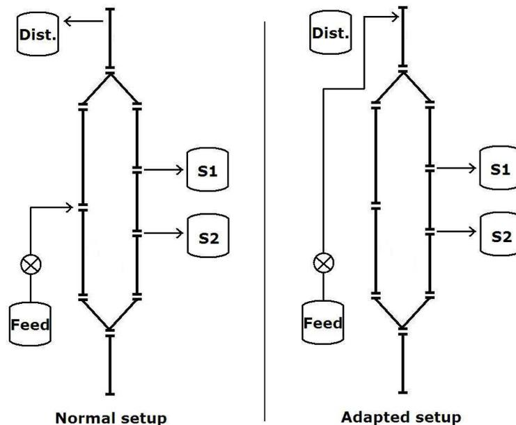
Figure 19: Adapted setup for the determination of the number of trays
