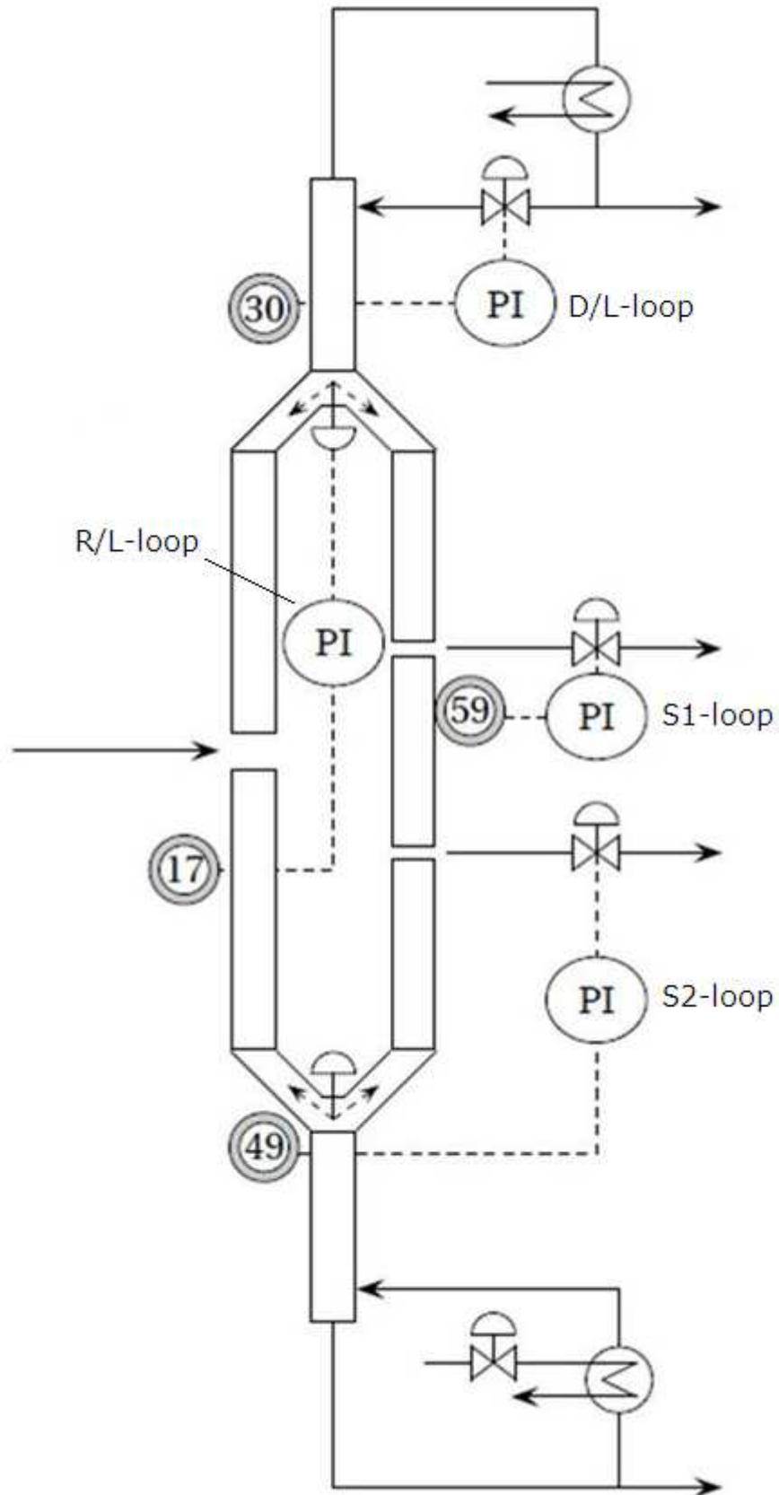
Figure 18: Temperature control loops
