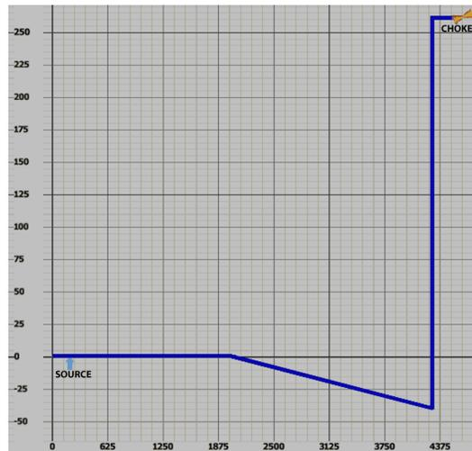
Figure 3.1: Illustration of the riser model with geometry
