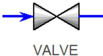
For the valves, there are three different sizing methods; Cv , Cg and k methods. I selected universal gas sizing method for my model; it uses the equation below;
