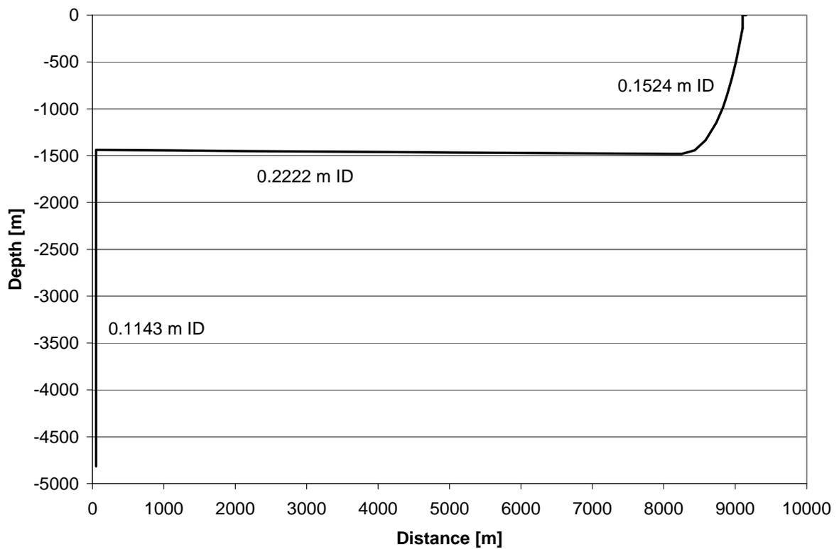
**Figure 2. Schematic description of well and pipeline profile.**
