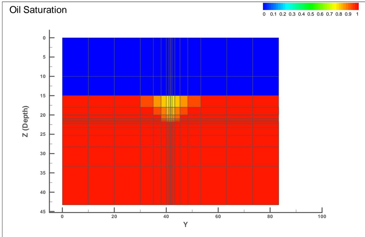
**Figure 11. Cross section of reservoir oil saturation just before the shut-in.**
