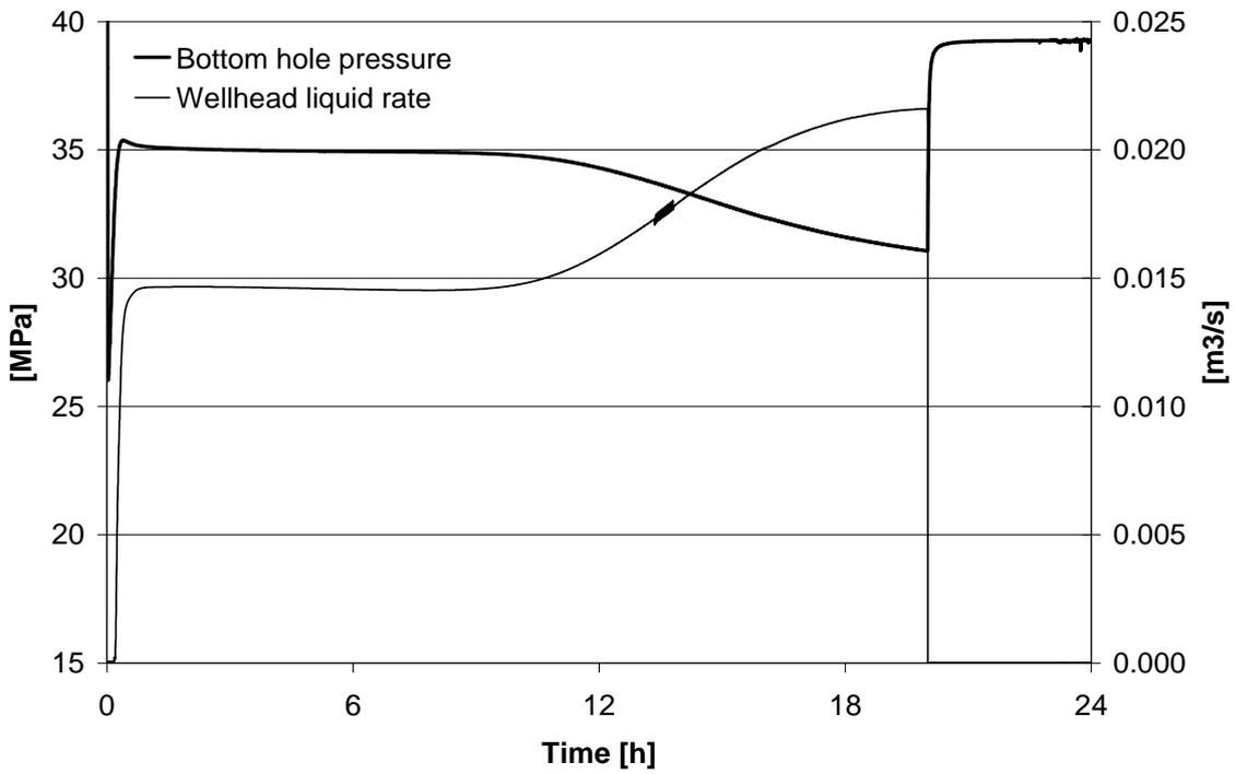
Figure 10. Bottomhole pressure and wellhead liquid rate.
