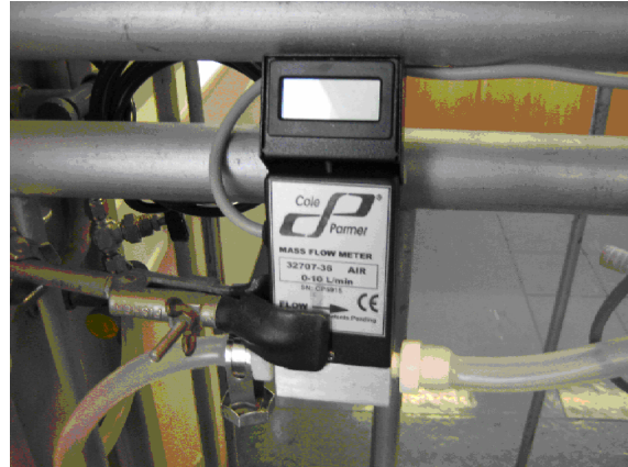
Figure 3.4 Flow rate meter, air.
