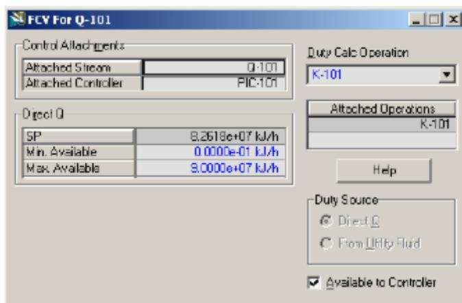
Figure 3.2: Specifying a maximum energy flow to a compressor
