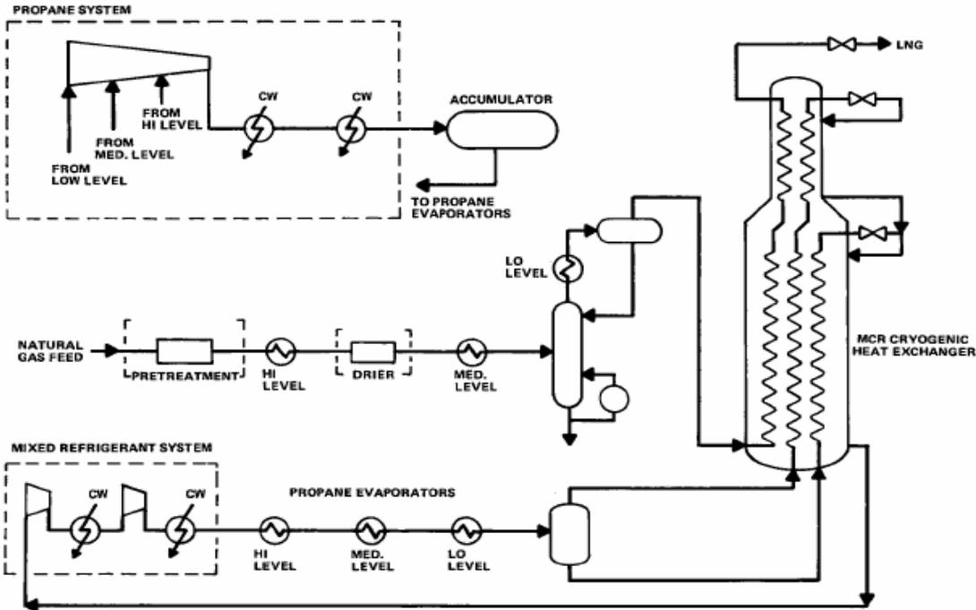
Figure 2.1: Schematic representation of a C3-MR process (from [7])
