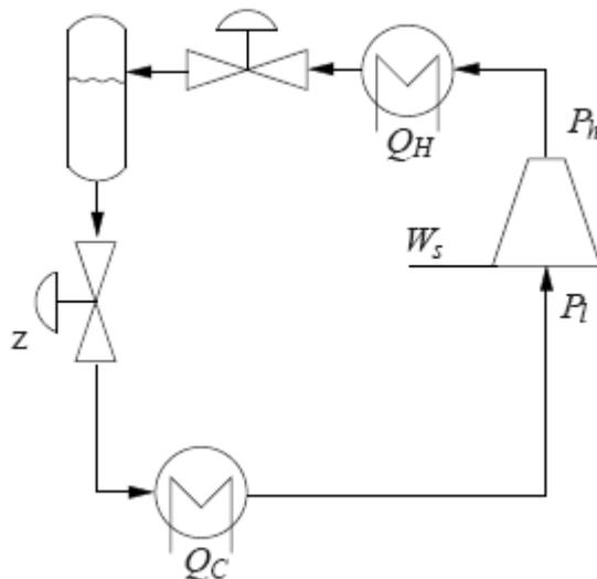
Figure 6.1: Typical positioning of level control valve and buffer tank in cooling cycle
