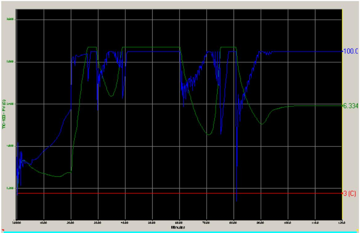
Fig. 5.17a: SP, PV and OP for TIC-103
