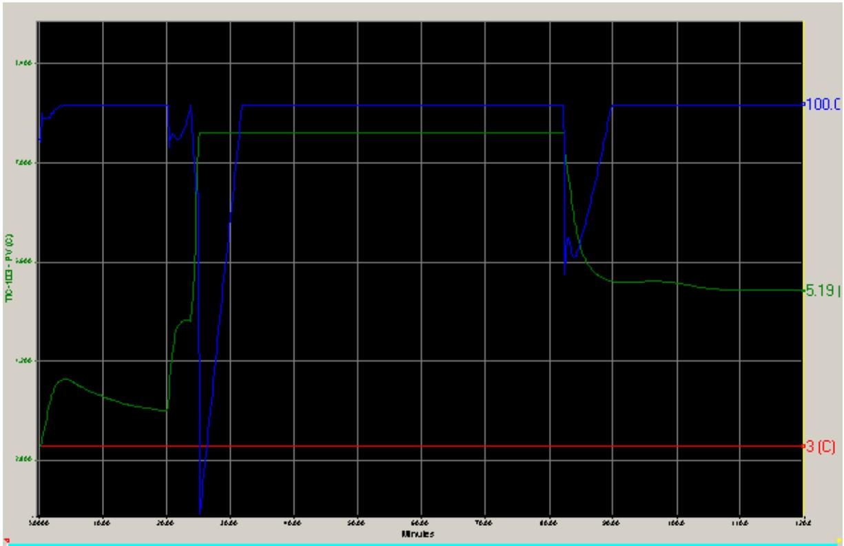
Figure 5.8a: PV, SP and OP for TIC-103. The output goes to saturation.
