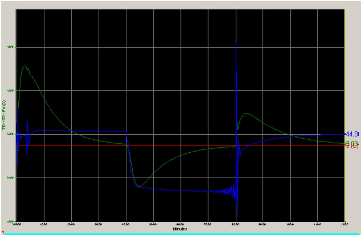
Figure 5.11a: PV, SP and OP for TIC-103 without cascade control
