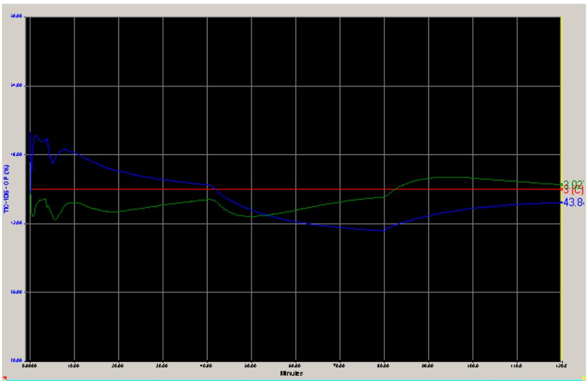
Figure 5.12 PV, SP and OP for TIC-106
