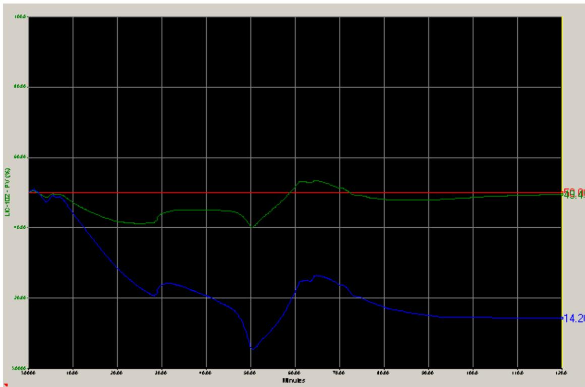
Figure 5.16 SP, PV and OP for LIC-102 (V-100 level control)
