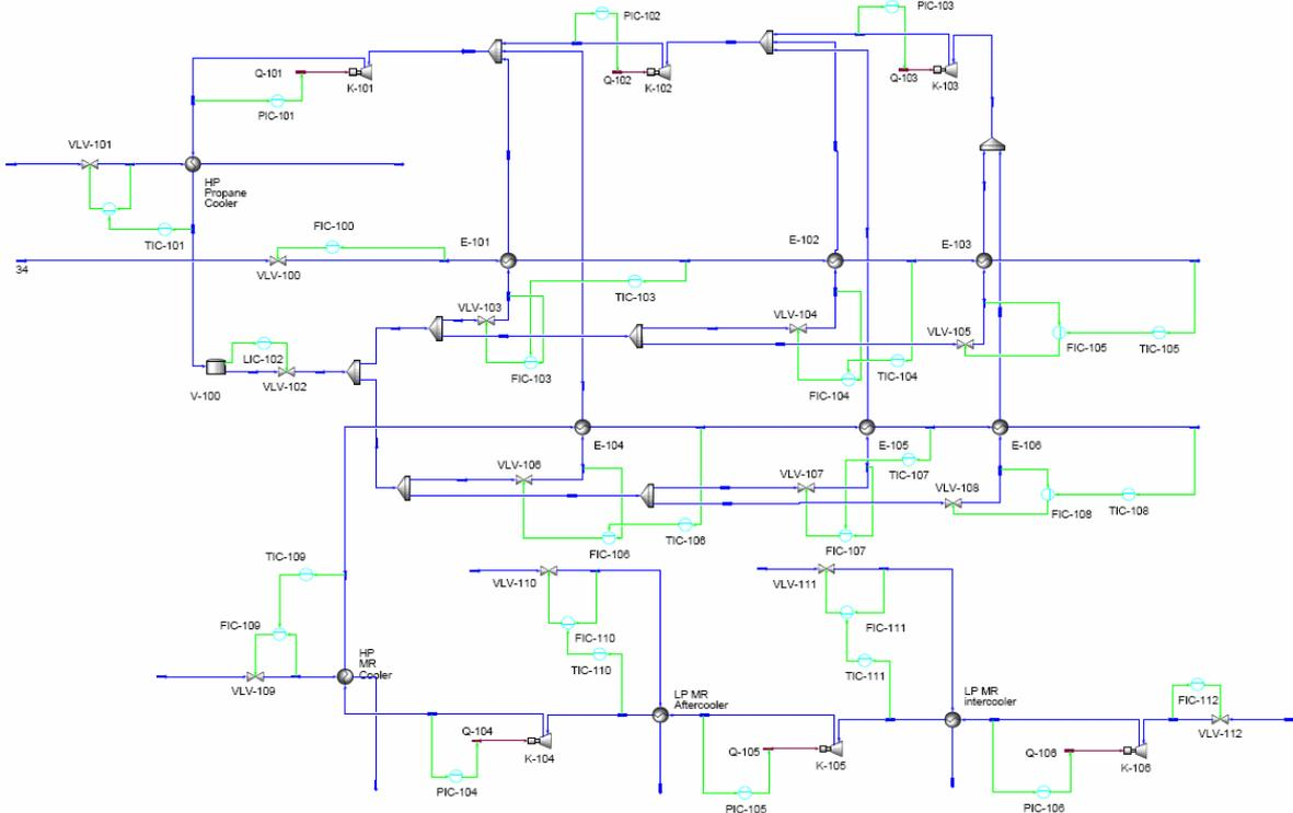
Figure 3.1: Flow sheet of the process as modelled in HYSYS, with controllers included
