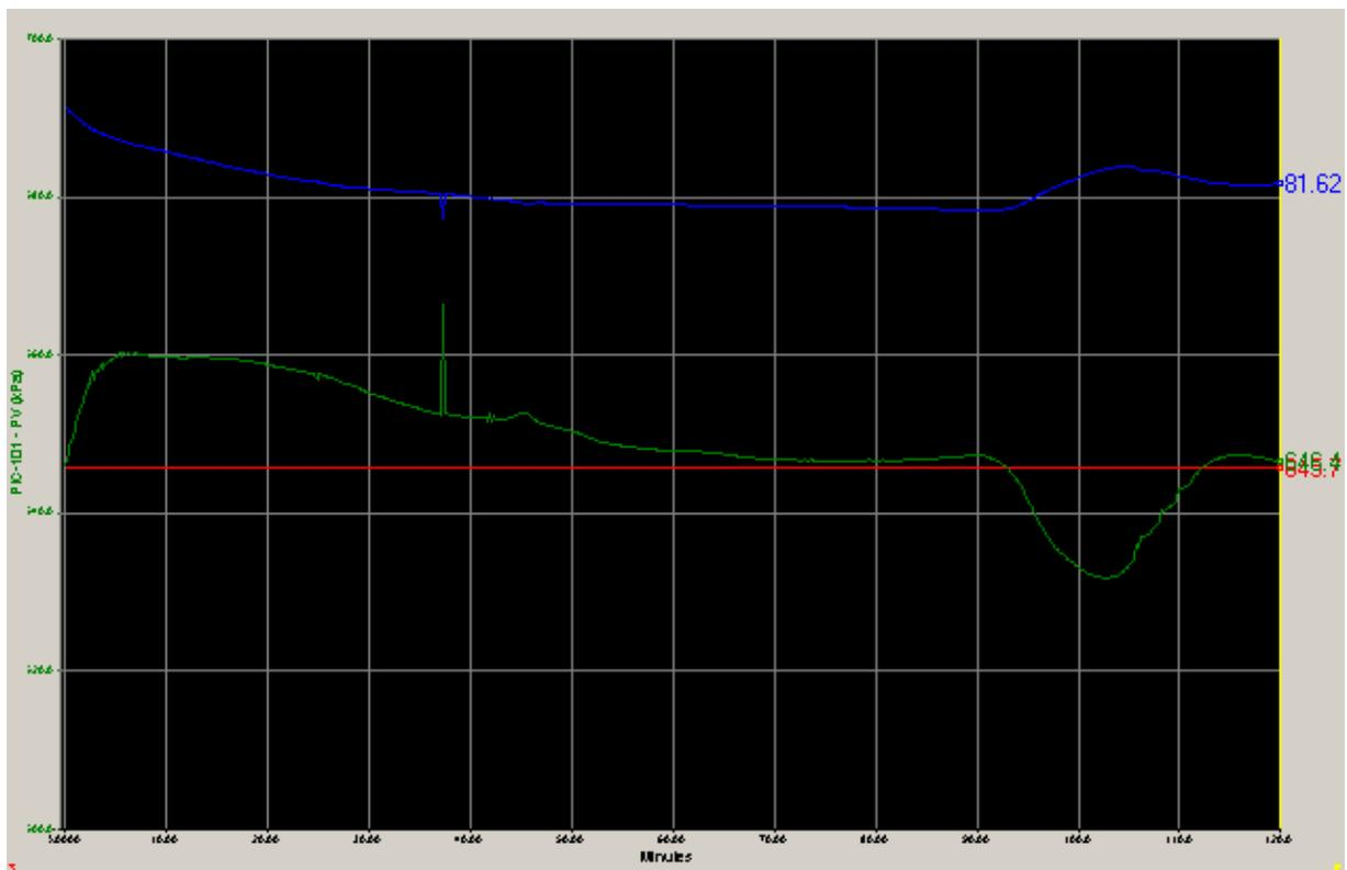
Fig. 5.3a: Pressure at outlet of K-101 (green), set point (red) and compressor power in % of max (blue)
