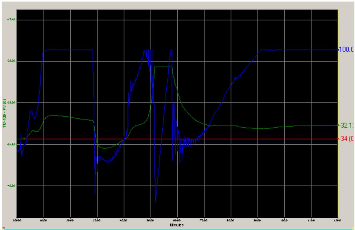
Fig. 5.17c: SP, PV and OP for TIC-105
