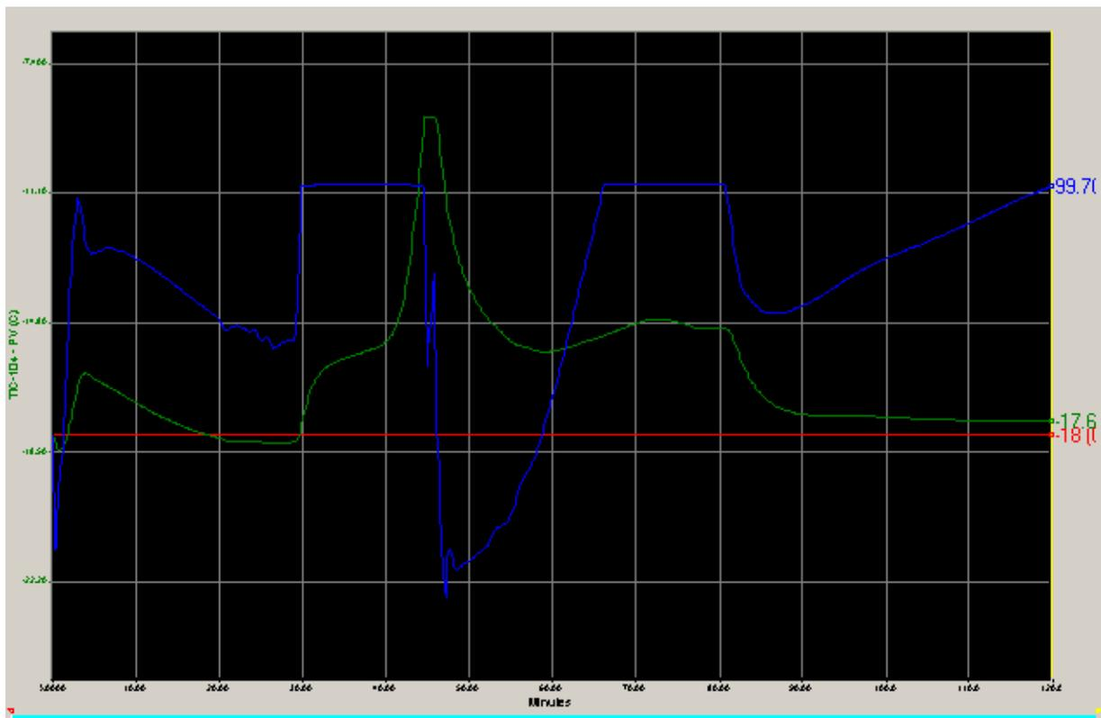
Figure 5.8c: PV, SP and OP for TIC-104
