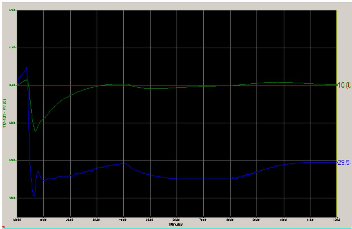
Figure 5.10: PV, OP and SP for TIC-101 (temperature after propane cooler)
