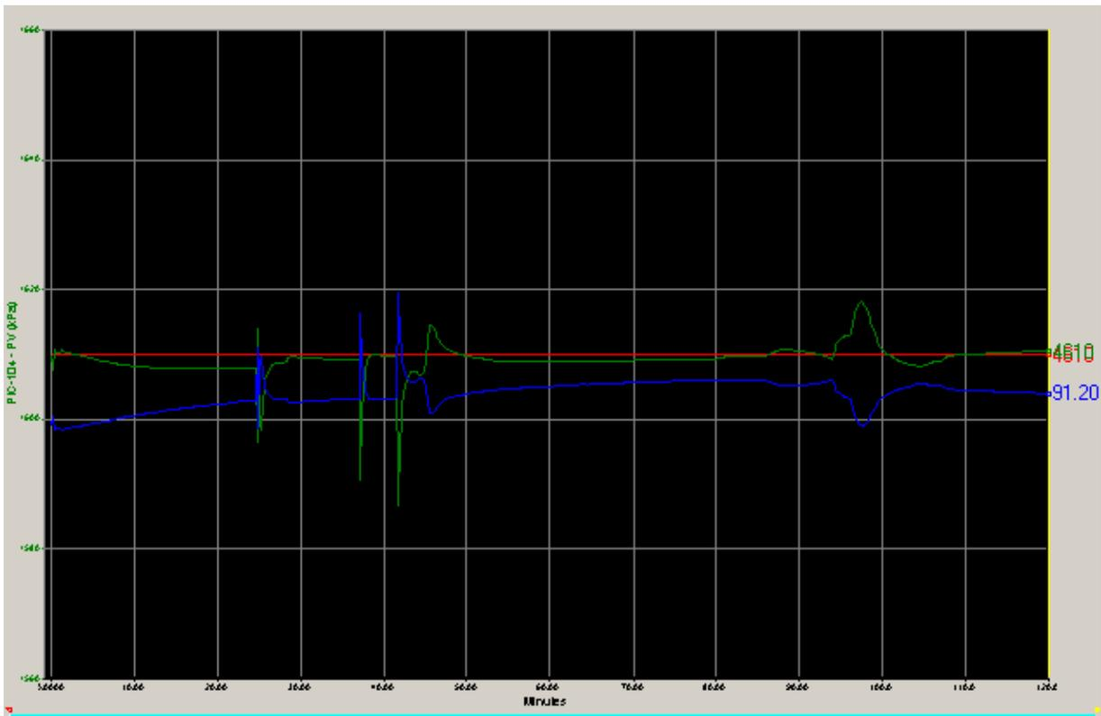
Figure 5.6: PV, SP and OP for PIC-104 (HP MR Compressor discharge pressure)
