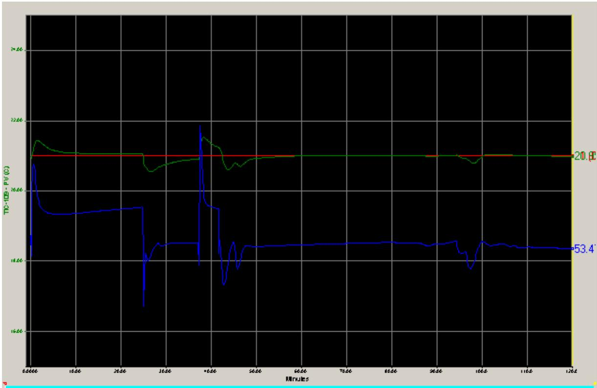
Figure 5.5: PV, SP and OP for TIC-109 (MR after cooler). OP varies between 45% and 75%.
