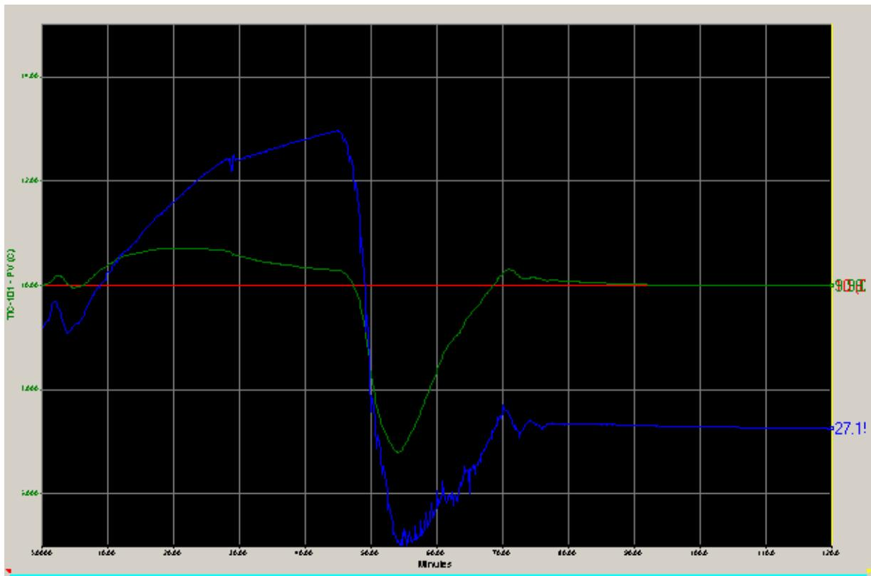
Figure 5.19: SP, PV and OP for TIC-101 (the propane condenser)
