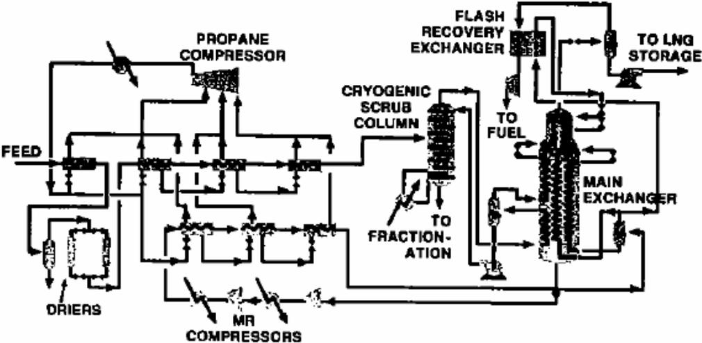
Figure 2.2 Schematic representation of a C3-MR process (from [2])
