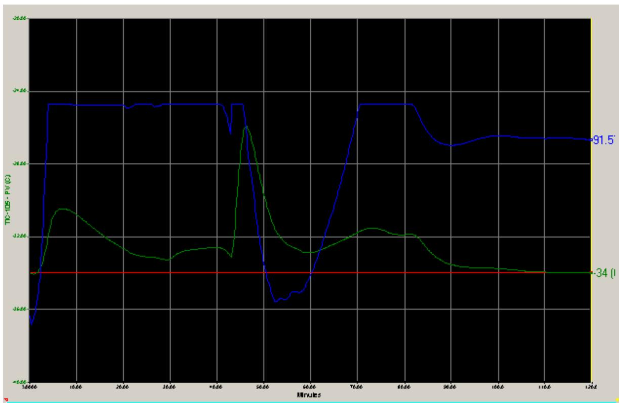
Figure 5.8d: PV, SP and OP for TIC-105
