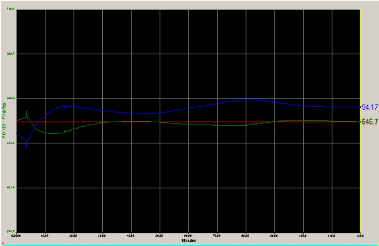
Figure 5.13: PV, SP and OP for PIC-101
