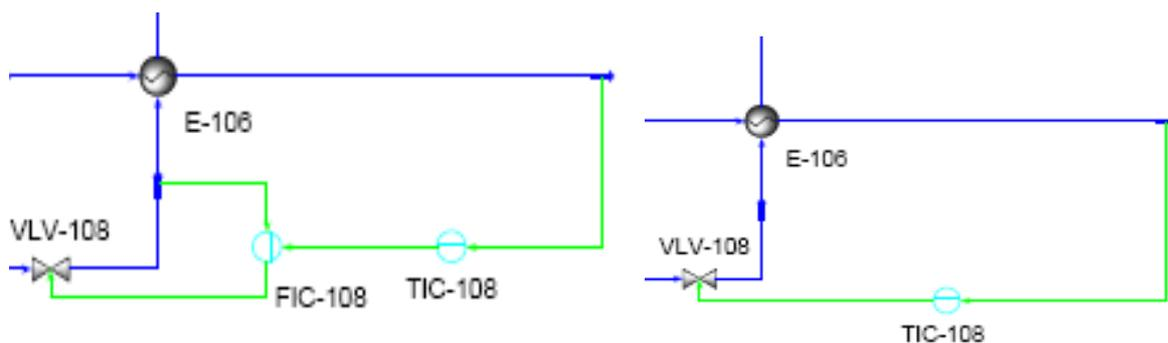
Figure 4.2: Control setup for heat exchanger (here: E-106). With cascade on the left, without on the right.
