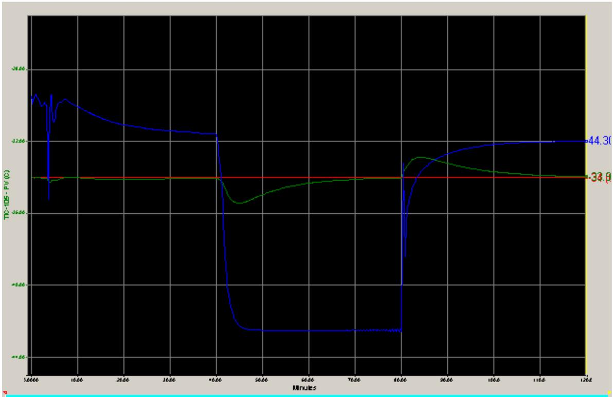
Figure 5.11c: PV, SP and OP for TIC-105
