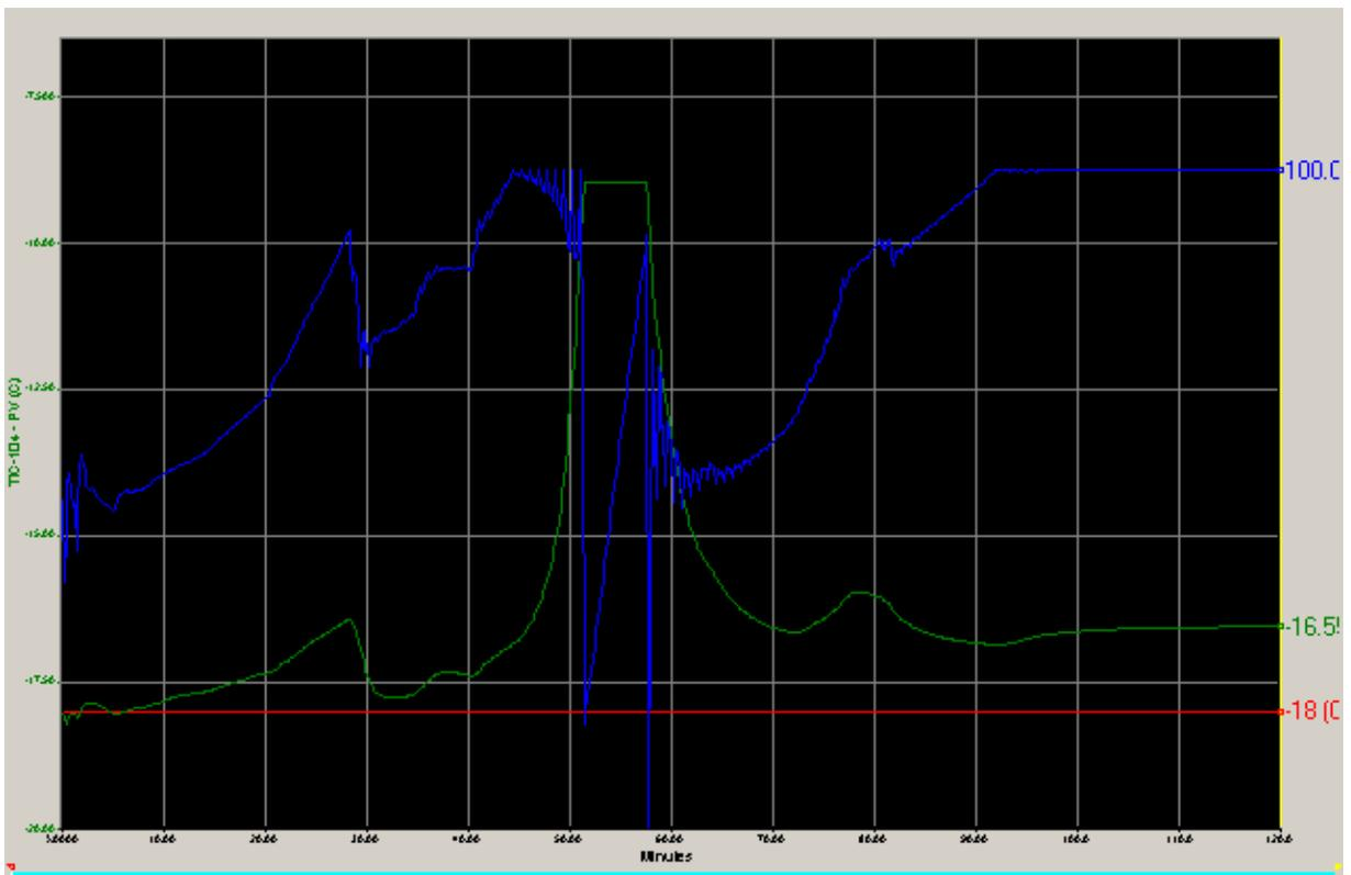
Fig. 5.17b: SP, PV and OP for TIC-104
