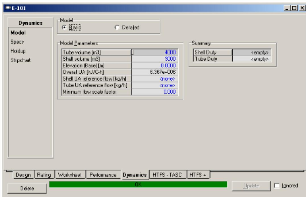
Figure 3.3: Specifying volumes in the basic heat exchanger model
