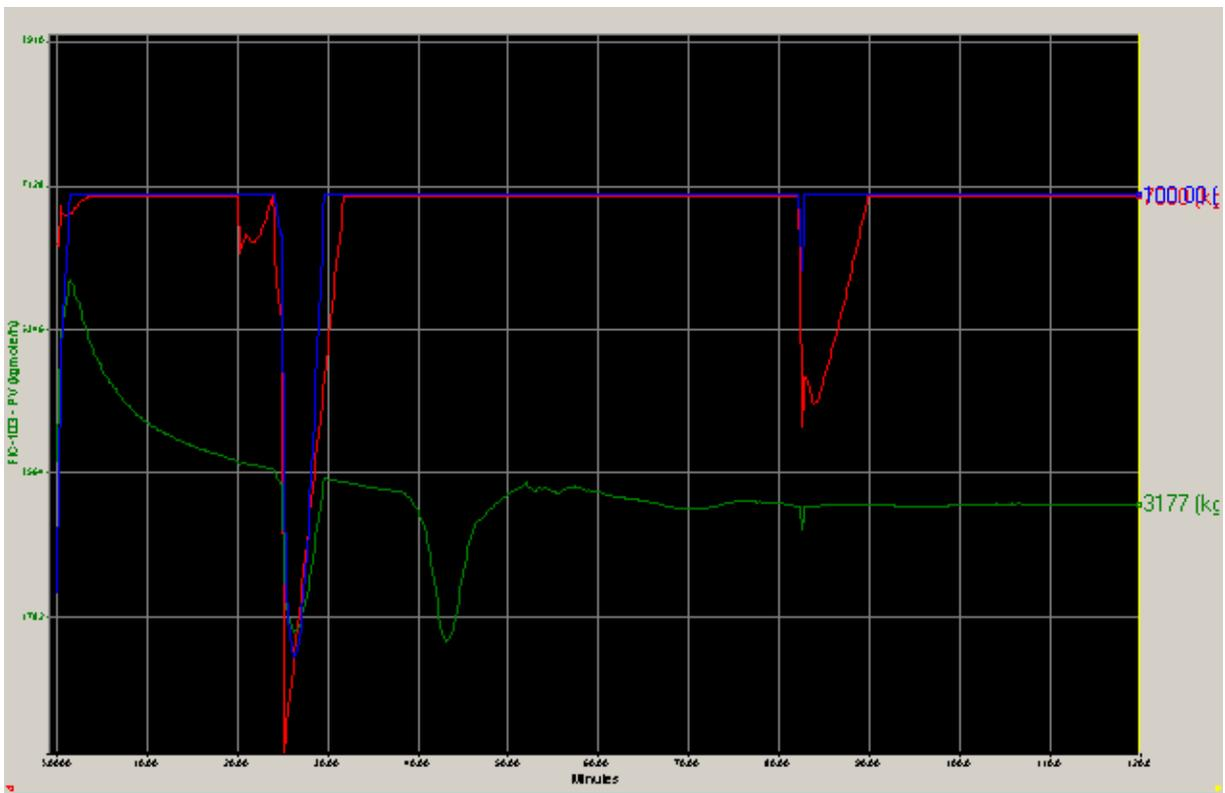
Figure 5.8b: PV, SP and OP for FIC-103 (the “slave” of TIC-103)
