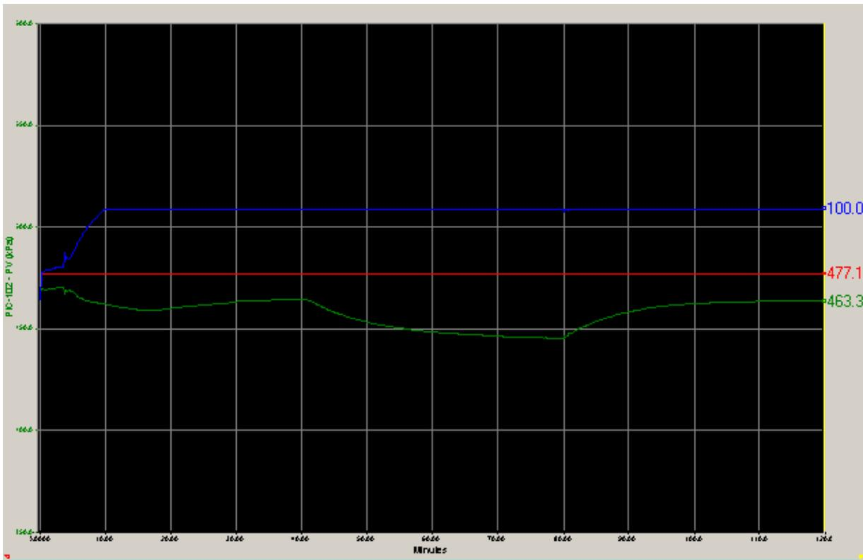
Figure 5.14: PV, SP and OP for PIC-102
