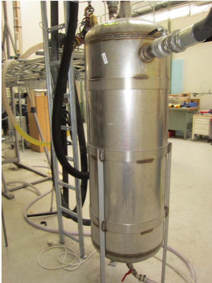
Figure 3.7: Air buffer tank
