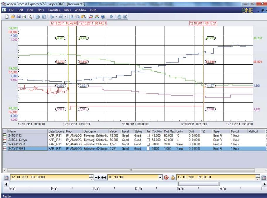
Figure A.2: Open loop step response in temperature controller at 91% feed rate with step magnitude of 1.0%. Process gain ( $k'$ ) and delay ( $\Theta$ ) are found to be 0.0421 and 2 min, respectively.
