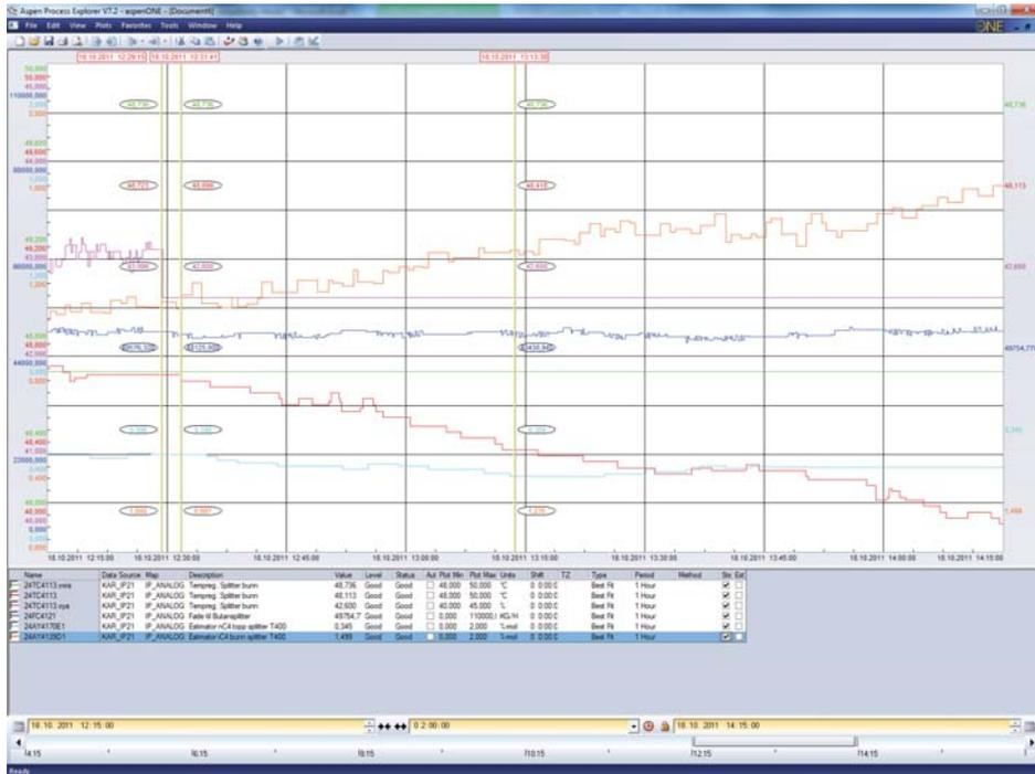
Figure A.1: Open loop step response in temperature controller at 66% feed rate with step magnitude of 0.5%. Process gain ( $k'$ ) and delay ( $\Theta$ ) are found to be 0.0267 and 2.43 min, respectively.
