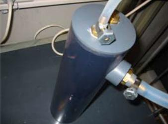
Figure 2.8 Buffer tank
