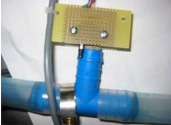
Figure 2.3 Pressure sensor
