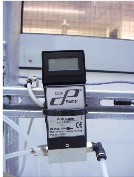
Figure 3.10: Gas flow rate meter
