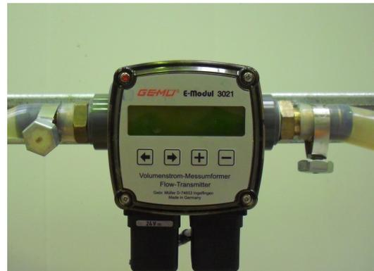
Figure 3.11: Water flow rate meter
