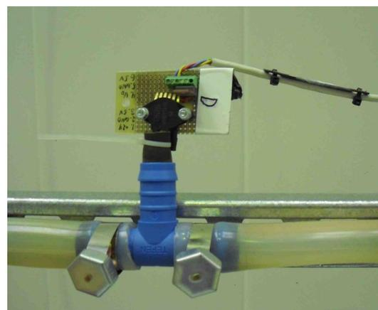
Figure 3.9: A pressure sensor
