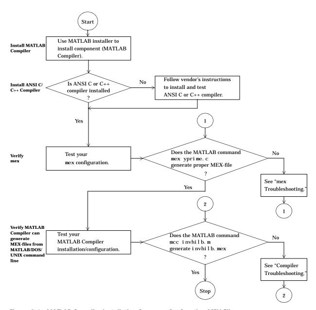
Figure 2-1: MATLAB Compiler Installation Sequence for Creating MEX-Files
