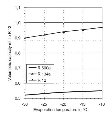
Figure 2: Volumetric capacity of R 600a and R 134a, relative to R 12, over evaporation temperature, at 55 °C condensing and 32 °C suction gas temperature, no subcooling
