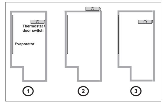
The main target of the safety precautions is to seperate rooms with refrigerant containing parts from rooms with switching elements.
